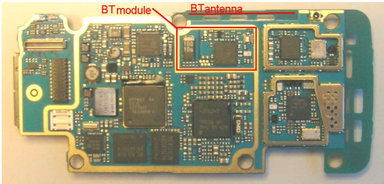
**3. MAIN PWB – TOP SIDE VIEW, BT UNDER SHIELD AS MARKED**
