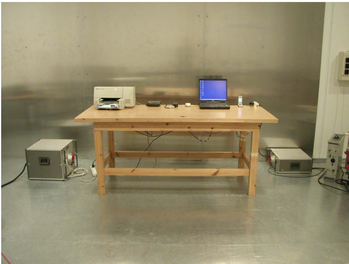
Photograph 1. AC power line conducted emissions test setup
