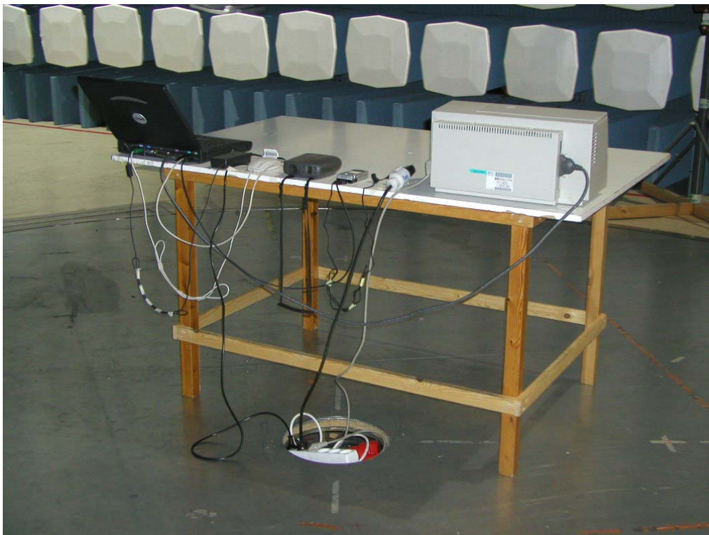
Photograph 2. Radiated emissions test setup
