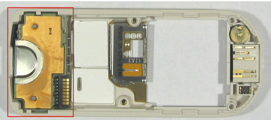
Marked in Red is Antenna both for BT and RF
