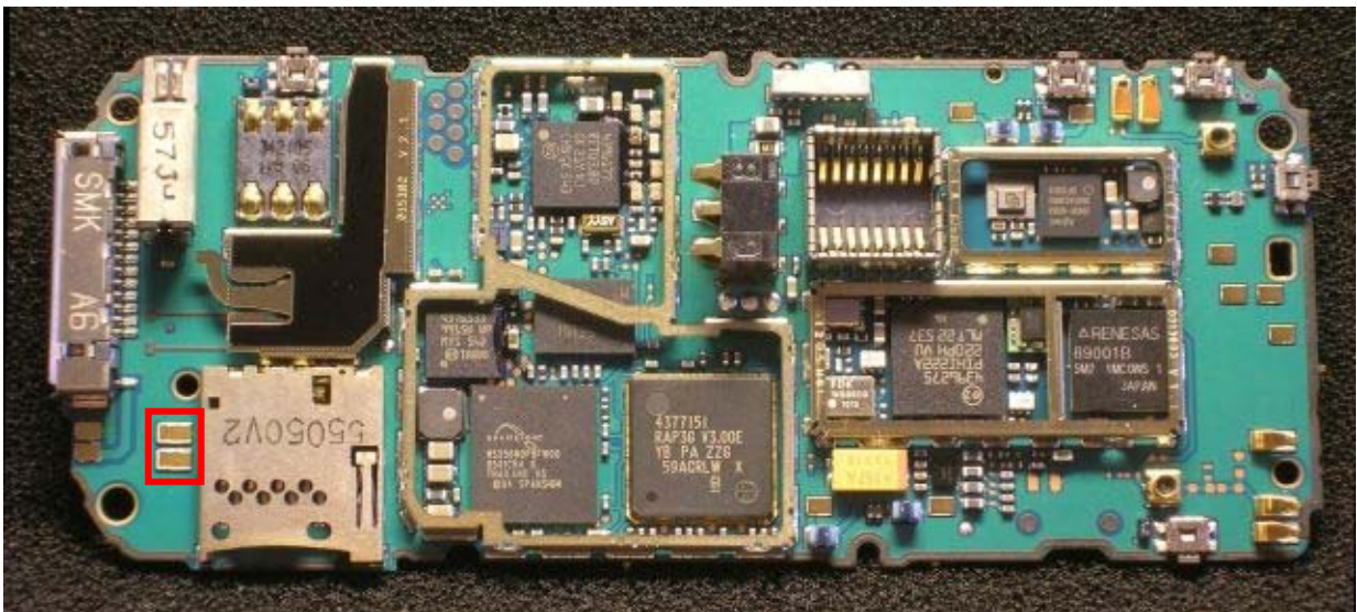
BATTERY Side (TOP side in parts list). Pads marked in red are BT antenna connection points. BT antenna is enclosed in phone's mechanics.
