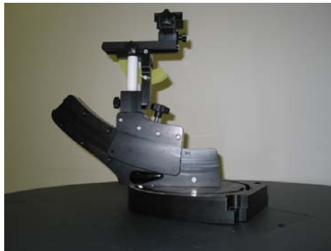
Device holder supplied by SPEAG
