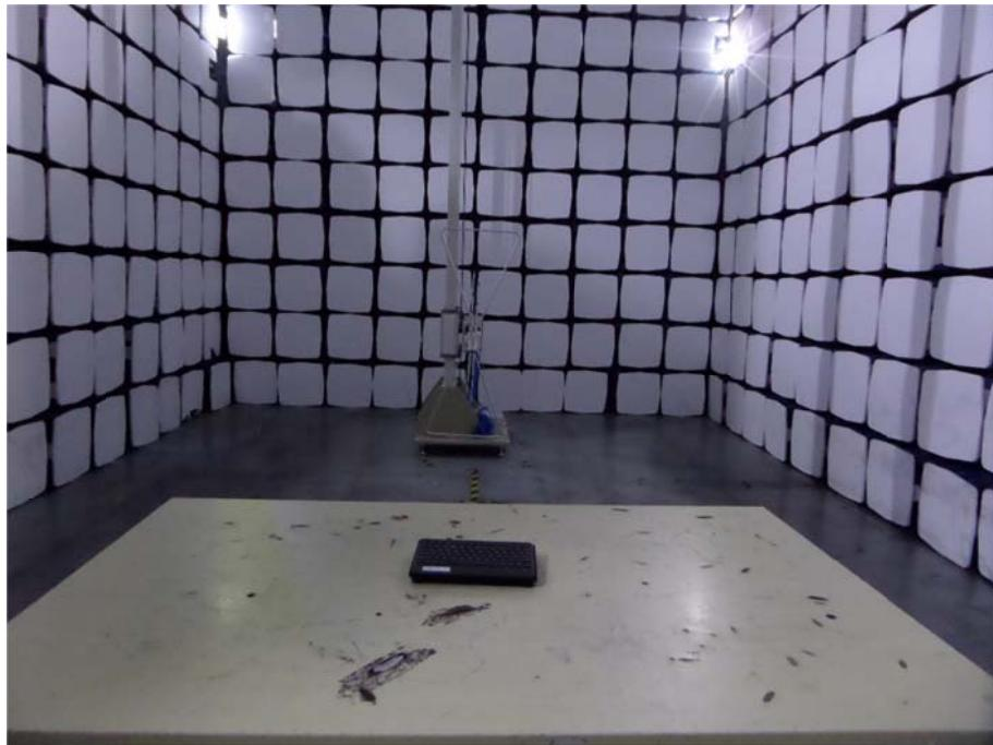
**Radiation Emission Test Setup (1GHz to 18GHz)**
