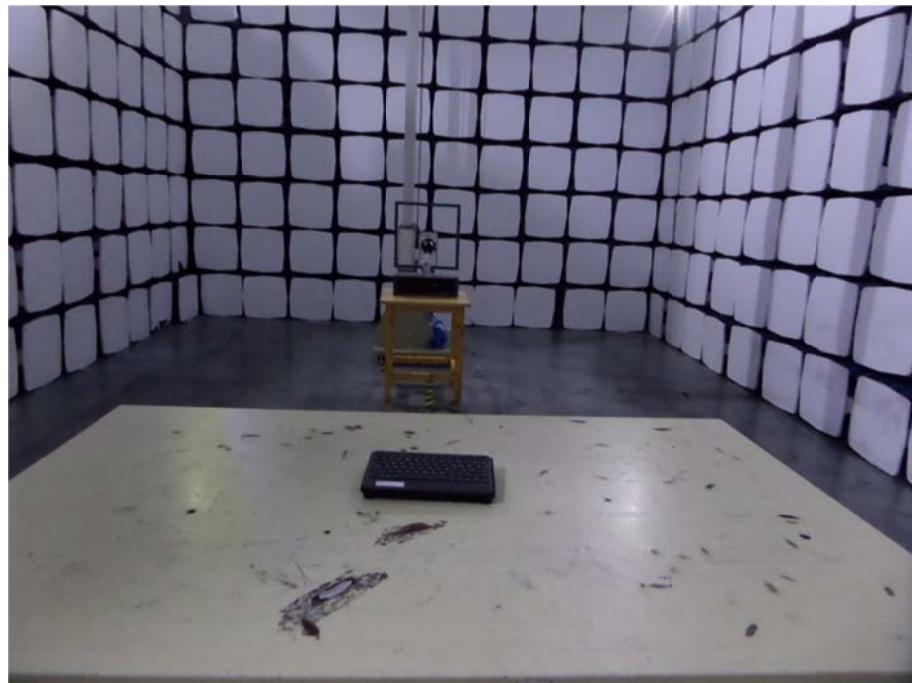
**Radiation Emission Test Setup (30MHz to 1GHz)**
