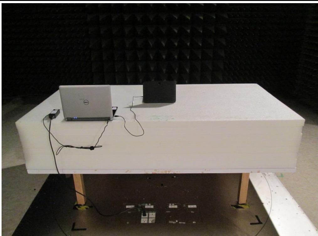
**Radiated Emission Above 1GHz Test**
