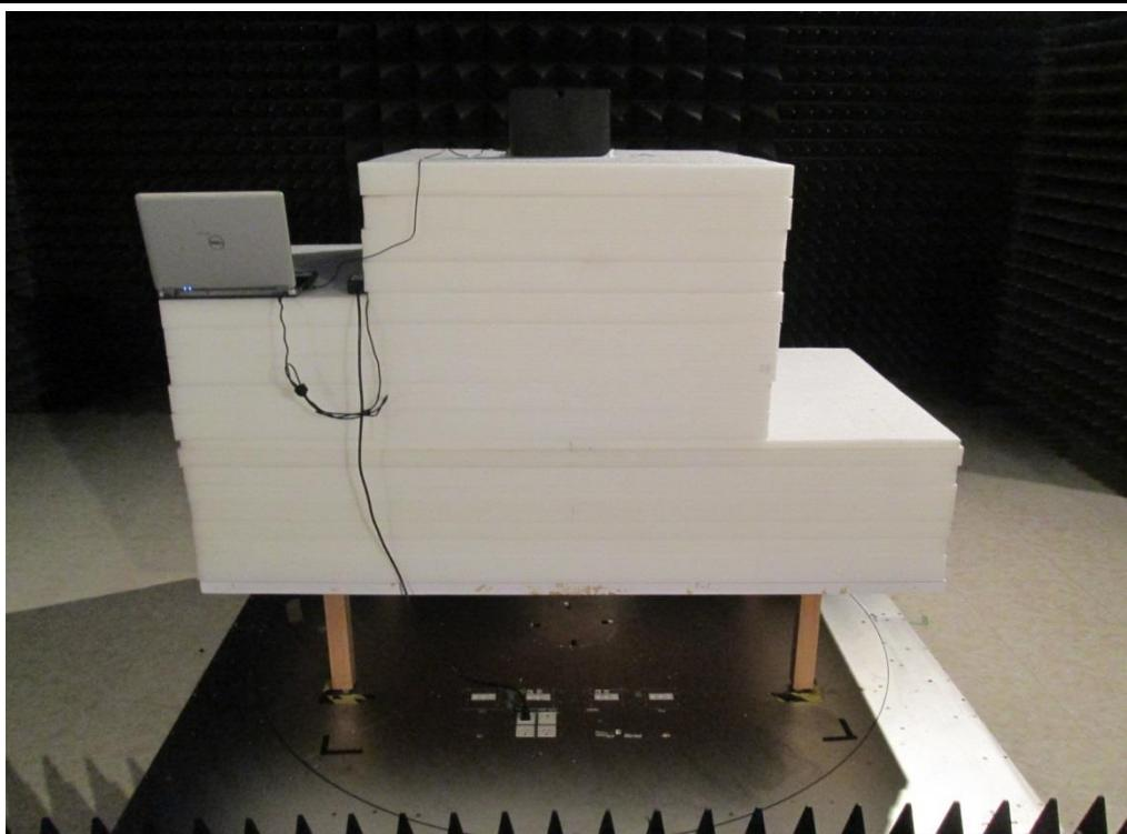
**Radiated Emission Above 1GHz Test**
