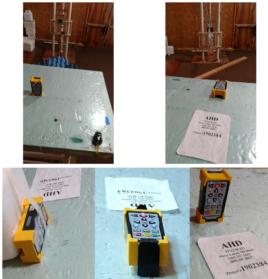
Figure 4: Radiated Emissions Test Setup Photograph(s).
