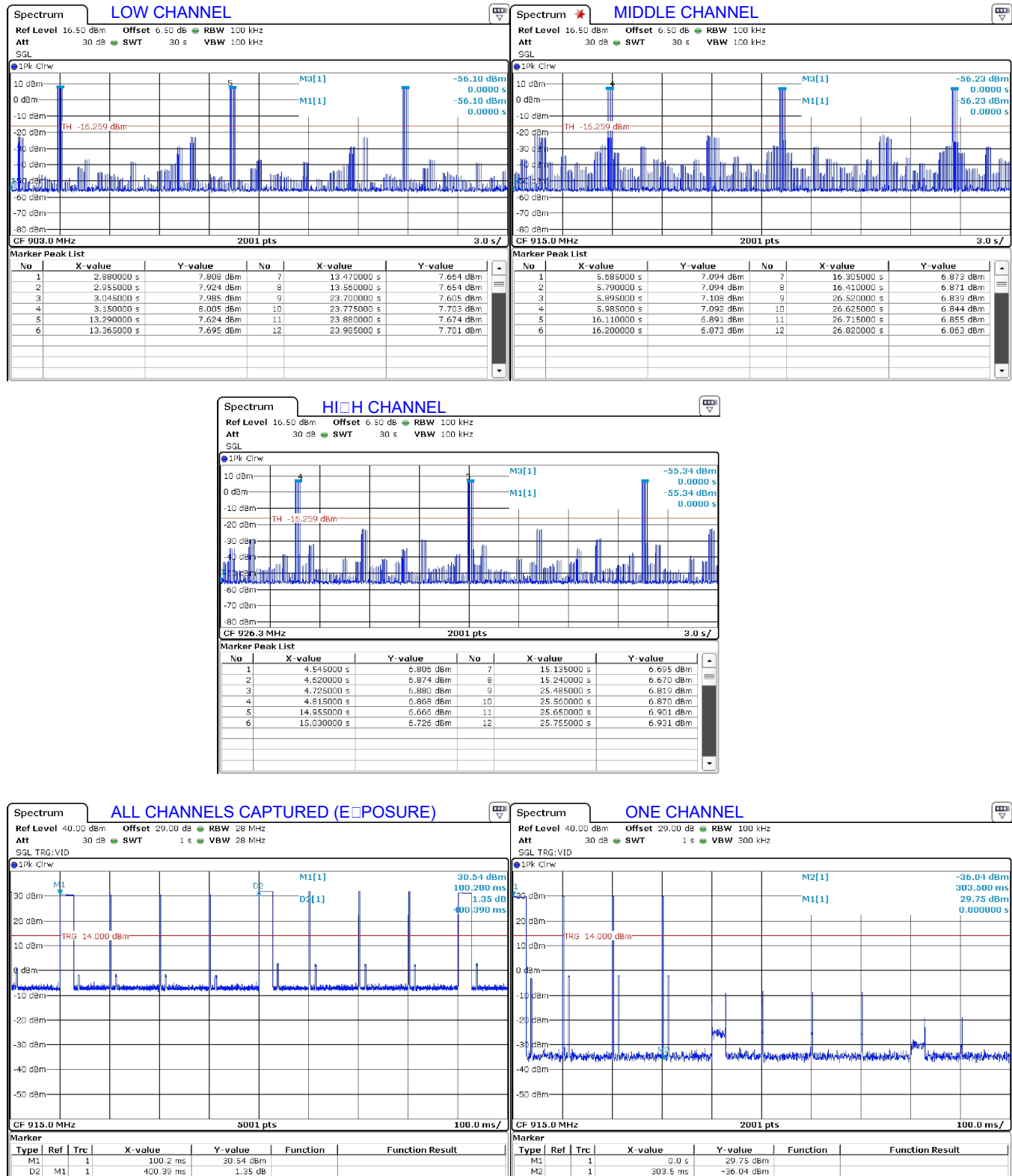
Figure 6: Example Plots of Duty Cycle and Channel Dwell Time.
