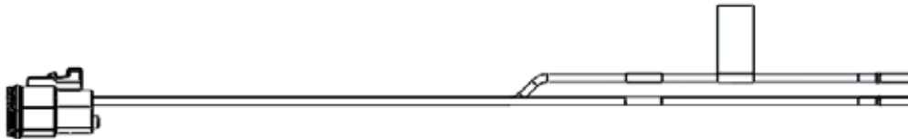
Cable D - P/N375440NT Valve Pigtail non-terminated harness for E14X/E16X valve actuator (optional)
