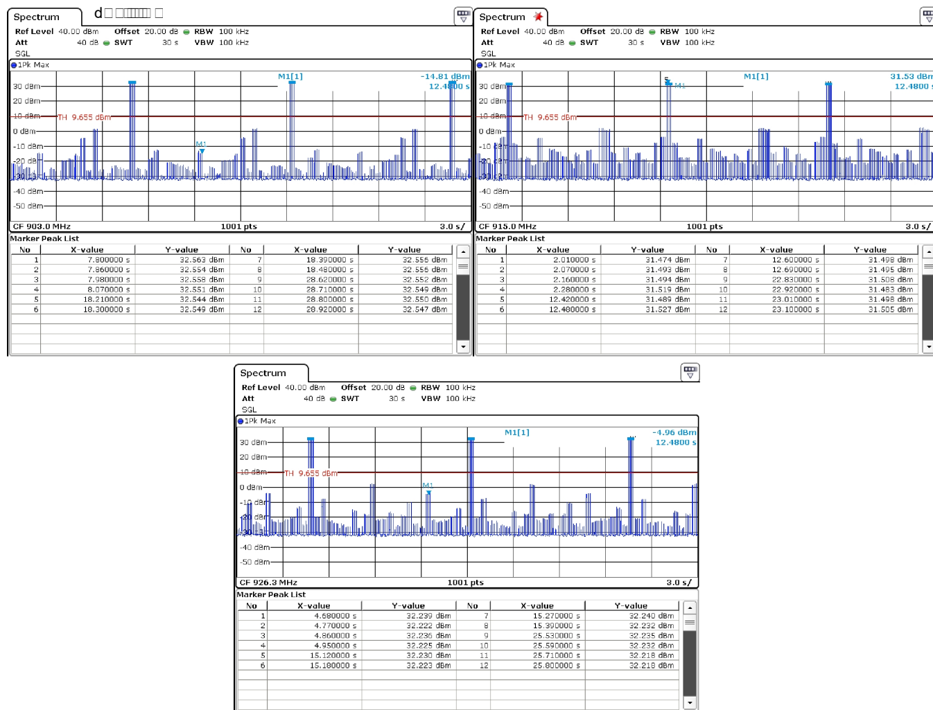
Figure 6(a): Example Plots of Duty Cycle and Channel Dwell Time.
