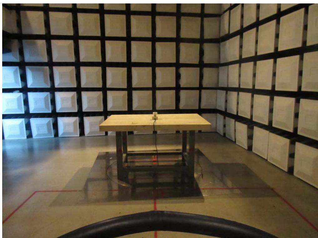
**Radiated Measurement Photos****30MHz to 1000MHz**
