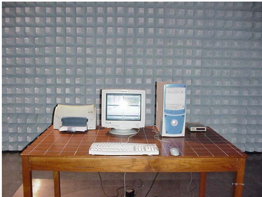
FIGURE 7. THE TEST SETUP PICTURE FOR RADIATED EMISSIONS TESTING
