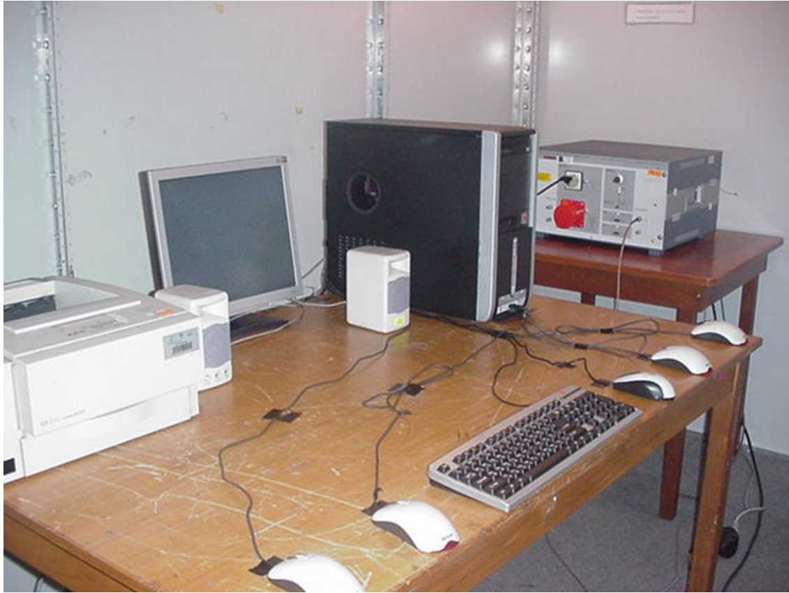
Figure 1-Conducted emission test set up
