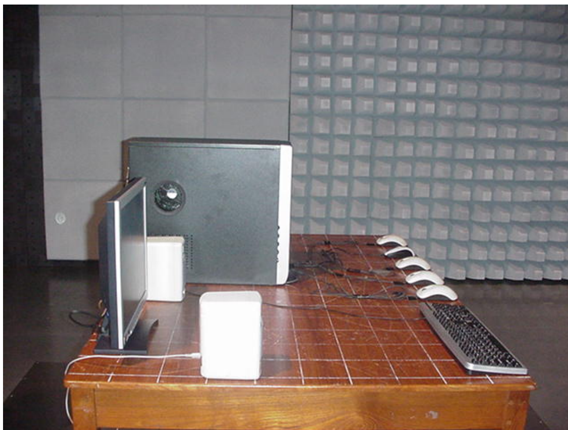
Figure 3-Radiated emission Test set up (side view)
