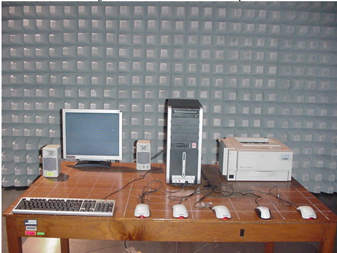
Figure 2-Radiated emission test set up
