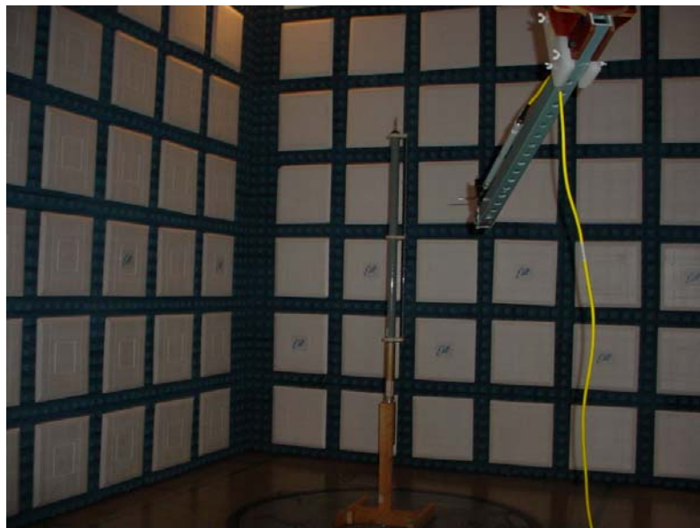
Test Setup For Measurement of Radiated Emissions Cyclone 900.7H Omni-directional Antenna Horizontal Polarity
