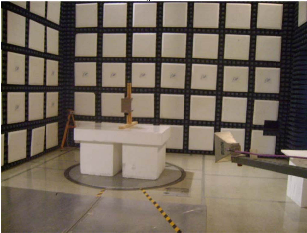
Test Setup for Radiated Emissions Horizontal Polarization
