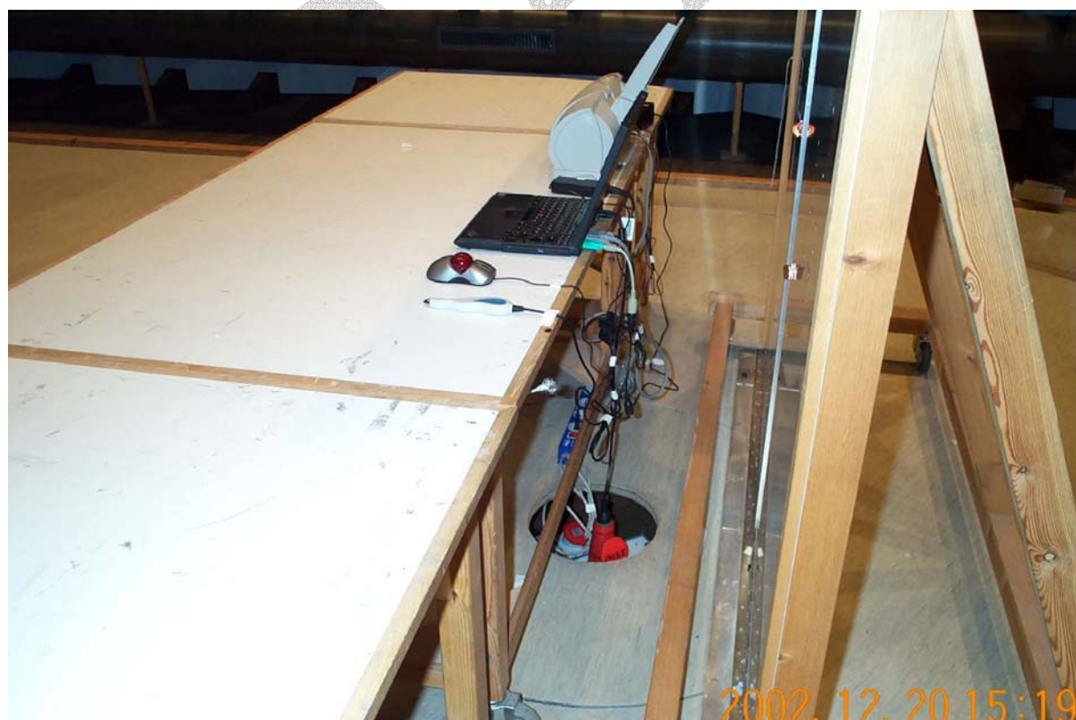
Photo A2.2 AC mains conducted emission measurement
