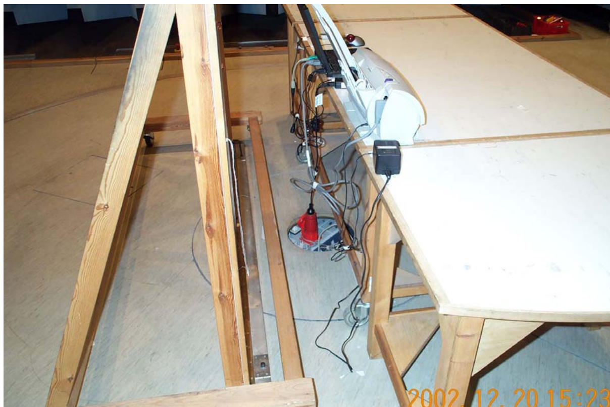
Photo A2.3 AC mains conducted emission measurement
