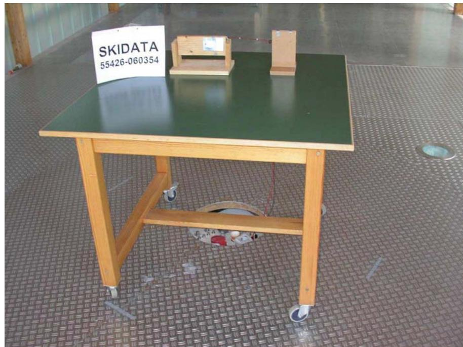
**Test setup for radiated emission measurement
