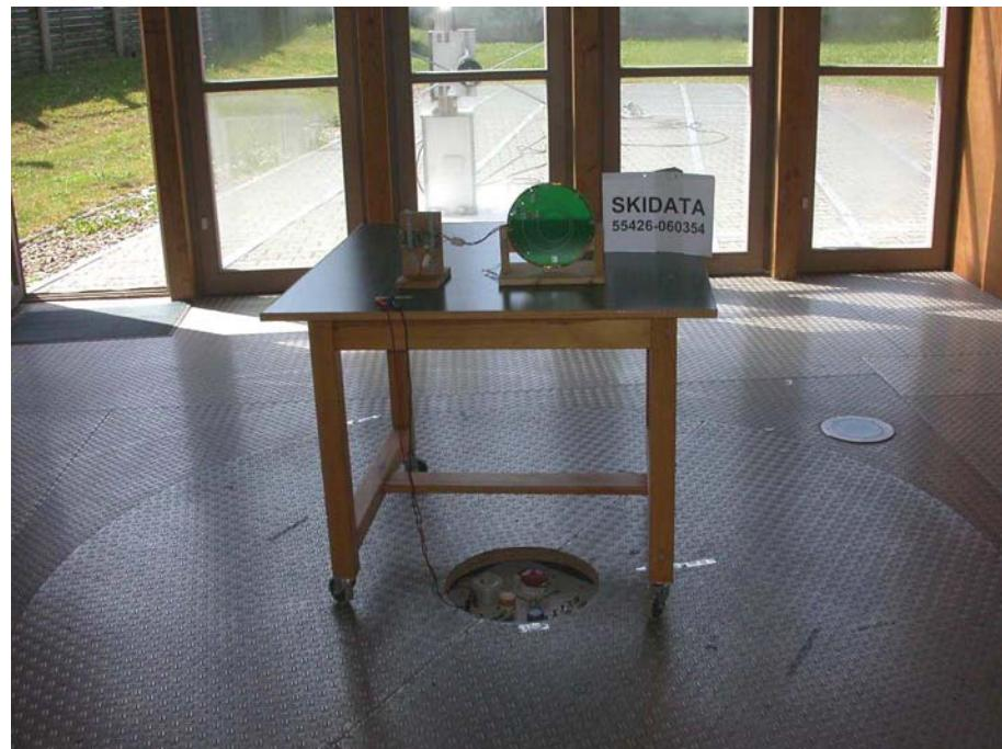
**Test setup for radiated emission measurement
