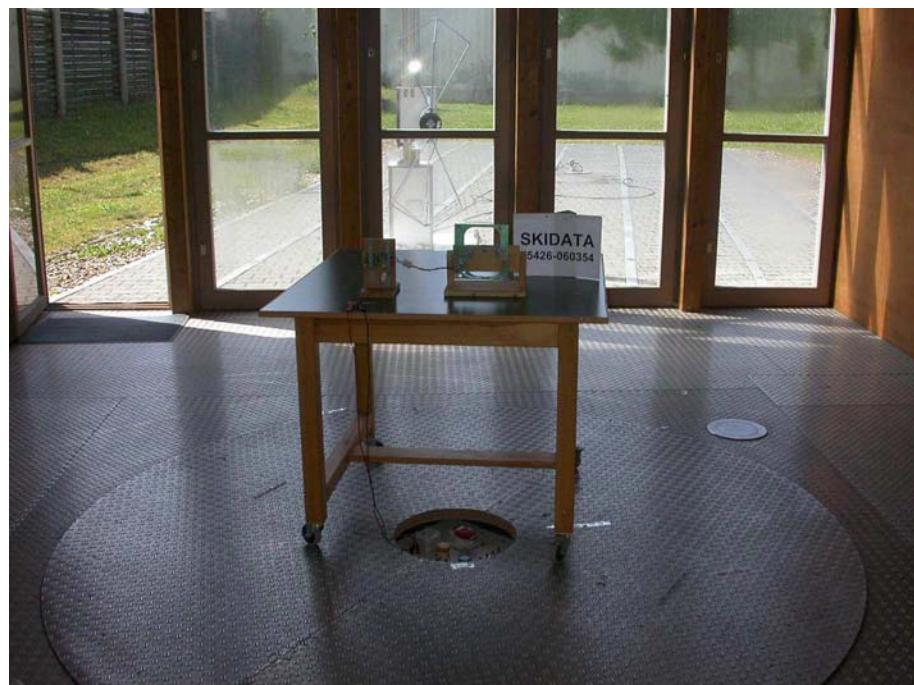
**Test setup for radiated emission measurement
