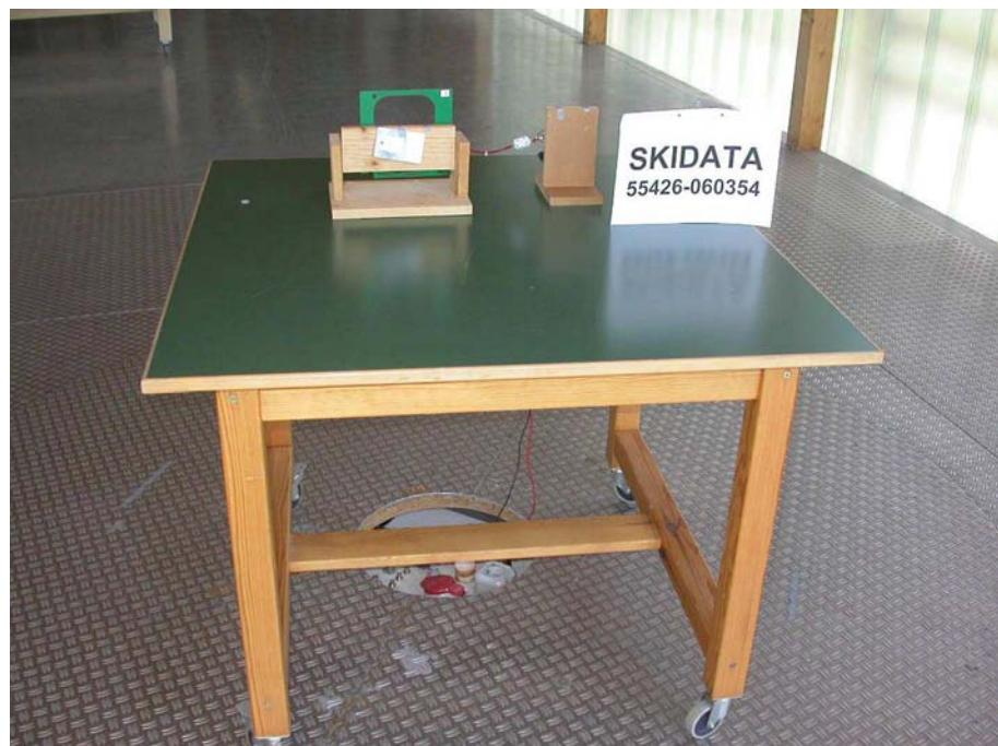
**Test setup for radiated emission measurement
