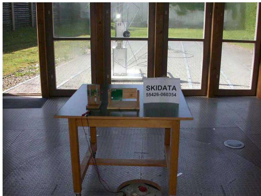
**Test setup for radiated emission measurement
