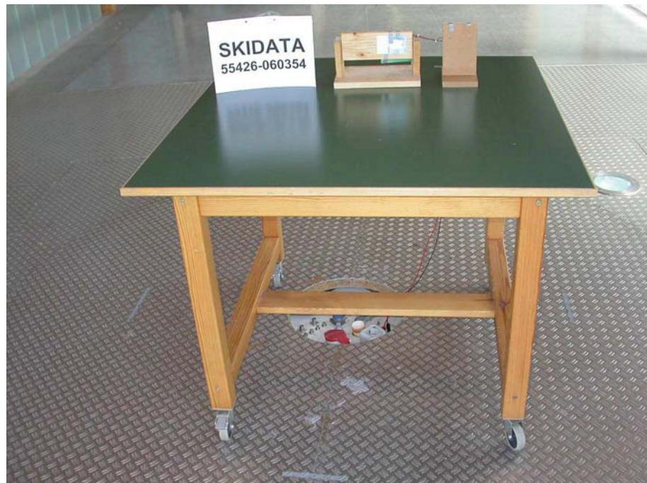
**Test setup for radiated emission measurement
