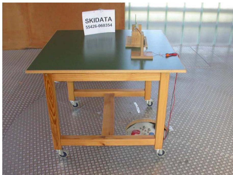
**Test setup for radiated emission measurement
