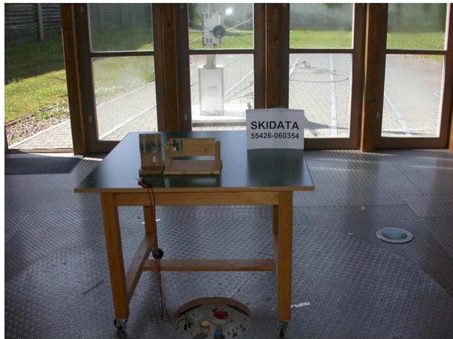
**Test setup for radiated emission measurement
