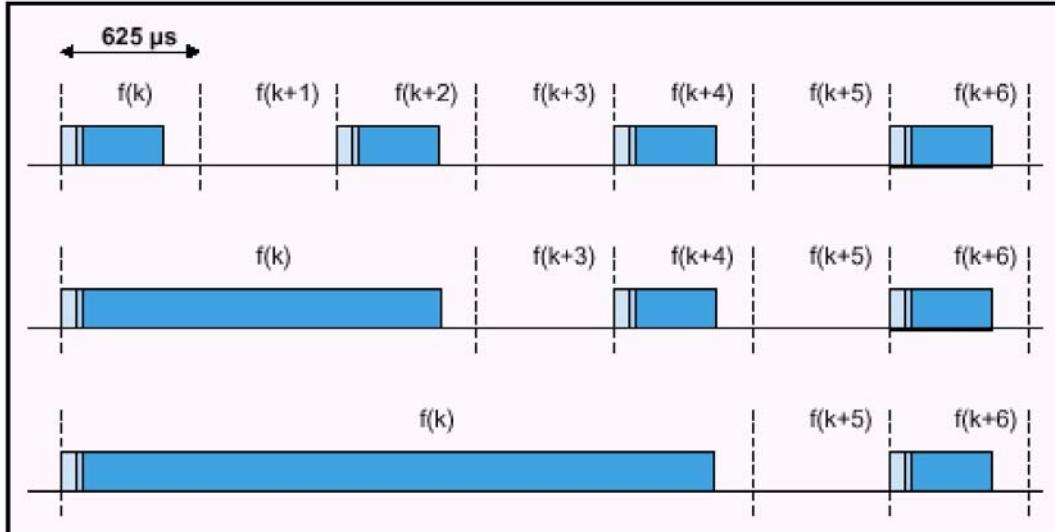
For DH5 packets the transmitter transmits across five 625 microsecond slots minus a guard band of 259 microseconds. The transmission is followed by a 625 microsecond receive slot. The transmission duty cycle (Tdc) for this case can be calculated as:
