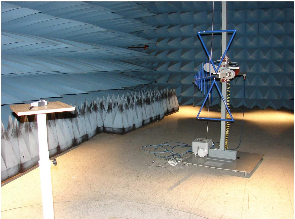
**TEST SET-UP FOR RADIATED MEASUREMENTS ABOVE 1GHz**
