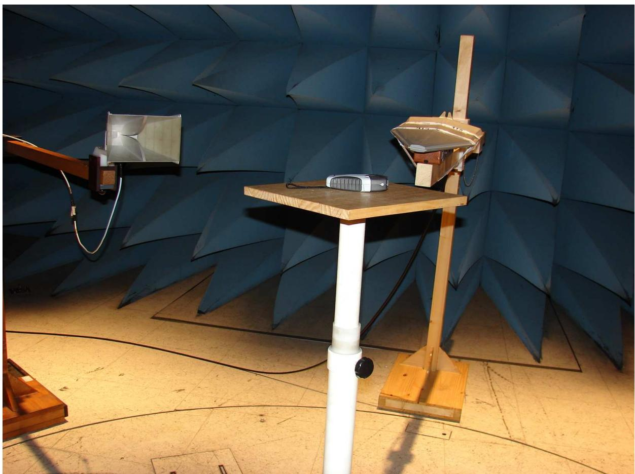
**TEST SET-UP FOR CONDUCTED MEASUREMENTS**
