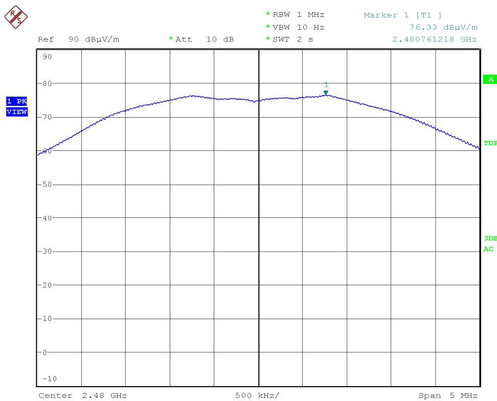
Note: The correction factor is already included in the spectrum analyzer as a transducer factor so that the marker shows directly the field strength level.
