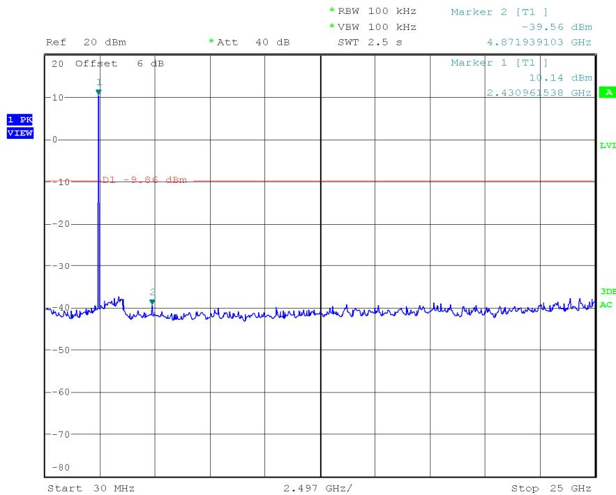
Note: The peak above the limits is the carrier frequency.
