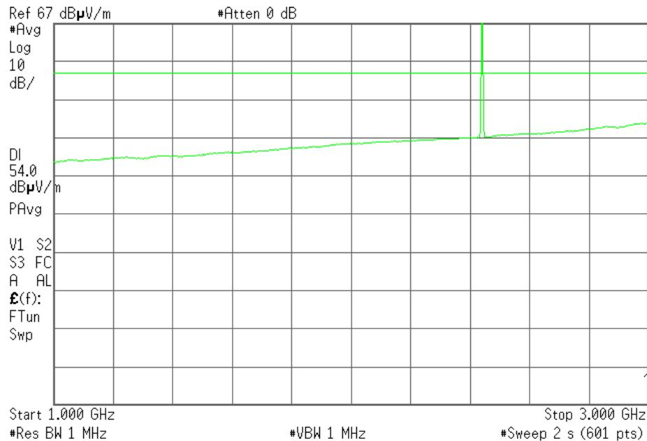
Note: The peak above the limit is the carrier frequency.
