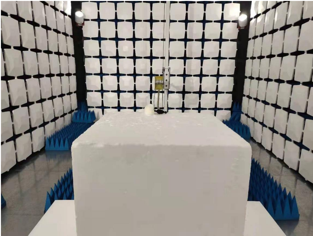
Above 1GHz for radiated emission test setup
