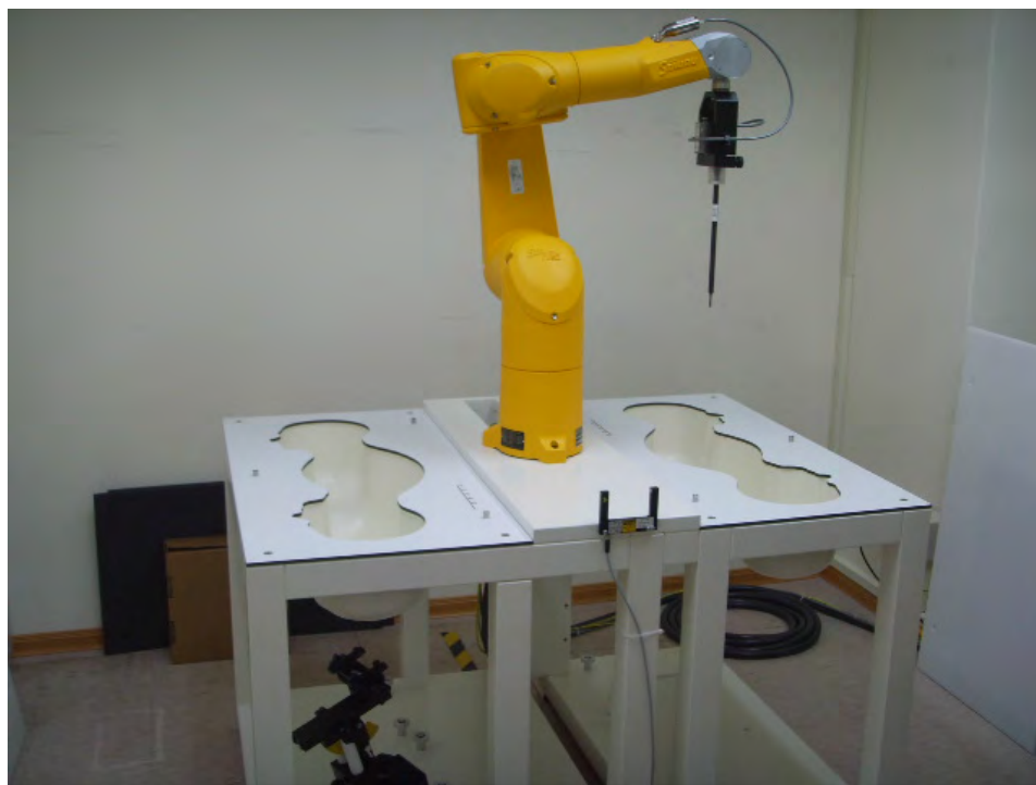
Fig.1 Photograph of the SAR measurement system
