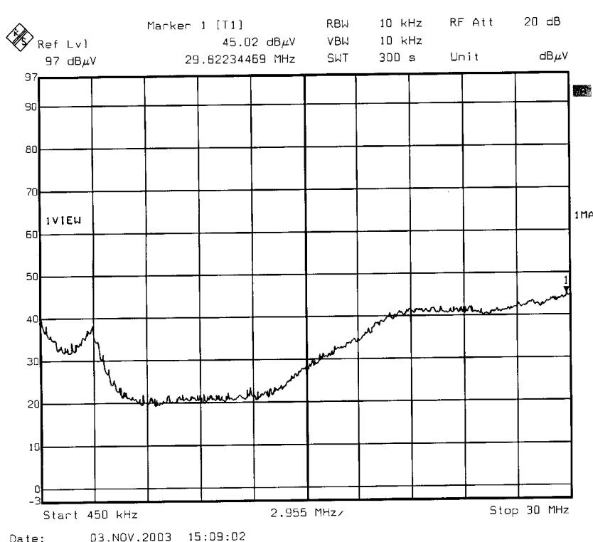
The plots of conducted emission tested with Commercial Electric power cord extension, M/N: EB-232-120-HPF was presented hereinafter as reference.
