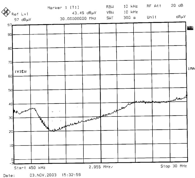
The plots of conducted emission tested with Commercial Electric power cord extension, M/N: EB-318-120-HPF was presented hereinafter as reference.
