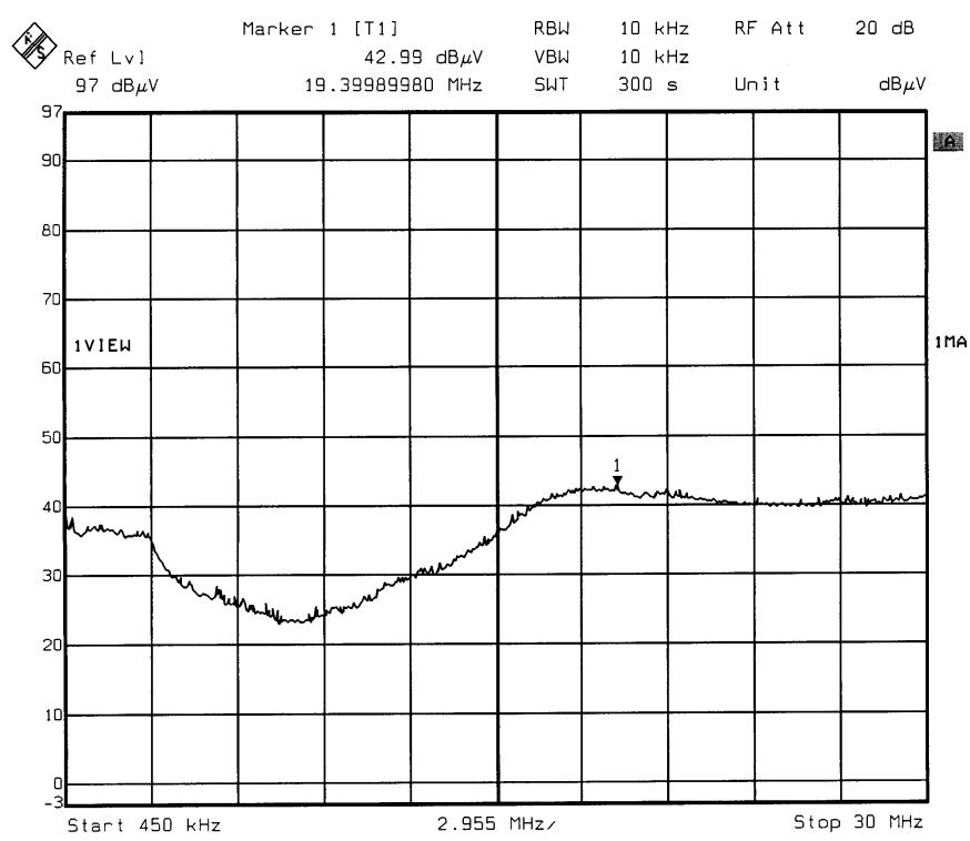
The plots of conducted emission tested with Commercial Electric power cord extension, M/N: EB-218-120-HPF was presented hereinafter as reference.
