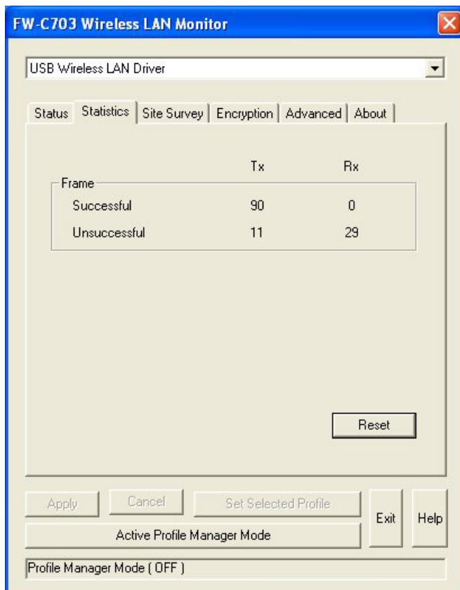
The **Statistics** utility allows you to view the statistic (Packets) information (Data Packets, Mgmt Packets, and Rejected Packets). To renew or update the list of statistics, click “**Reset**”.
