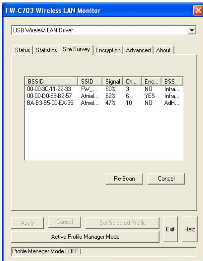
The **Site Survey** utility allows you to scan all the channels to locate all the APs (Access Points) within the range of your WLAN Adapter. When an/Various AP(s) are located, information regarding the BSSID and SSID, signal strength and channel where the AP operates, whether or not WEP encryption is used, and the operating mode is shown. Click “**Re-Scan**” to update the list. You may stop rescanning by press the “**Cancel**” button.
