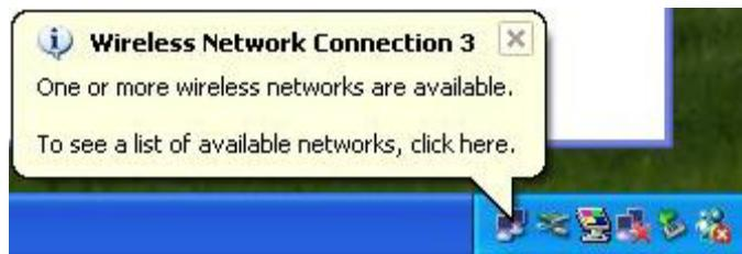
3. Click on the message and the “Automatic Wireless Network Configuration” will display automatically. You may click “Connect” button to connect with an available Access Point.
