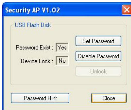
**Notice:** After you finish the configuration, you need to remove the device from USB port first and then plug in again to make configuration take effect.
