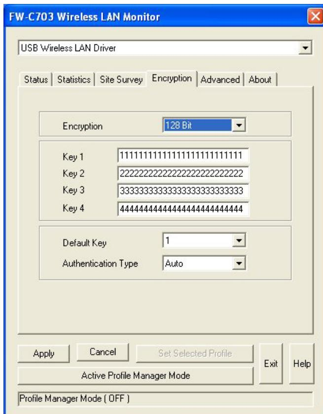
To prevent unauthorized wireless stations from accessing data transmitted over the network, the **Encryption** utility offers highly secure data encryption by allowing you to set four different WEP keys (must be the same for the participating wireless stations) and specify which one to use. To set encryption:
