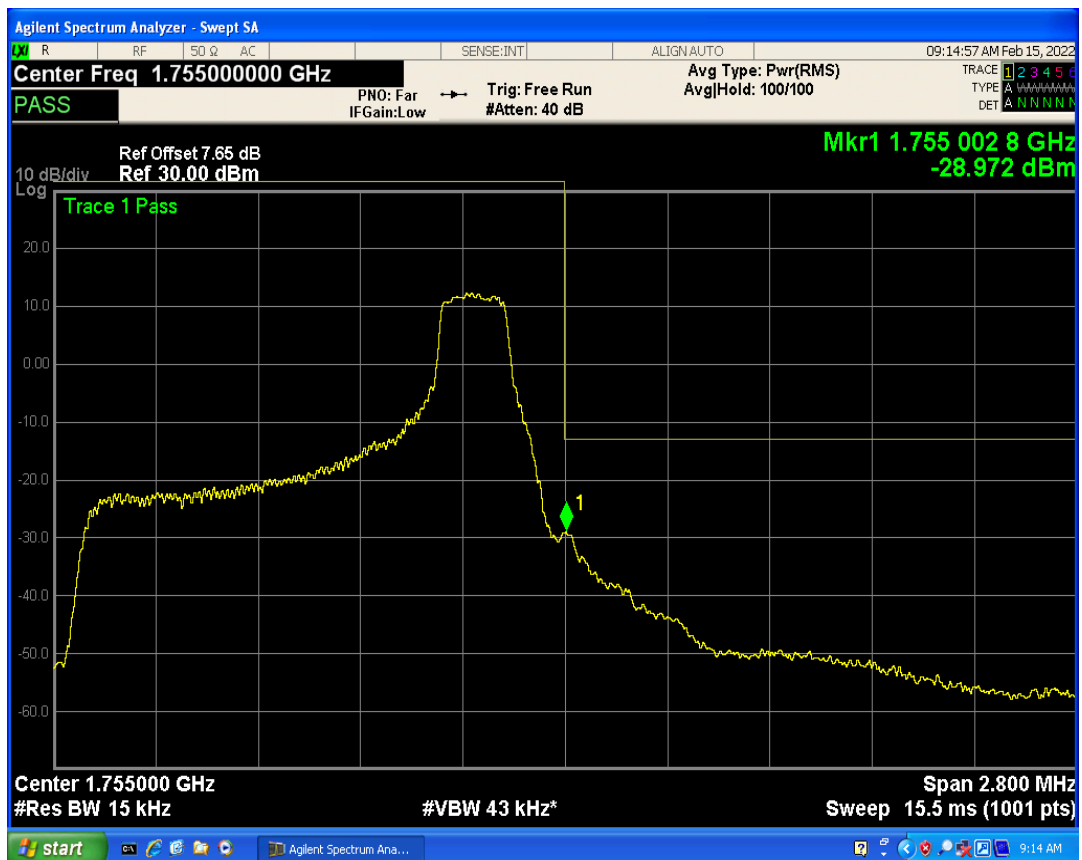
Band4 QAM16 BW=1.4MHz Channel=20393 RB Size=1 Position=#0
