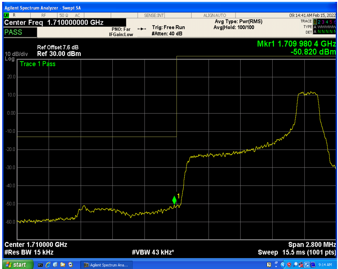
Band4 QAM16 BW=1.4MHz Channel=19957 RB Size=6 Position=#0
