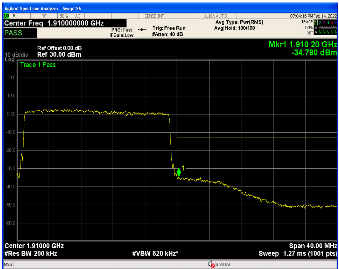
Band4 QPSK BW=1.4MHz Channel=19957 RB Size=1 Position=#0
