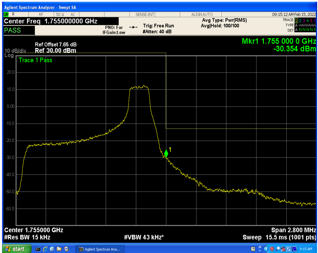
Band4 QAM16 BW=1.4MHz Channel=20393 RB Size=6 Position=#0
