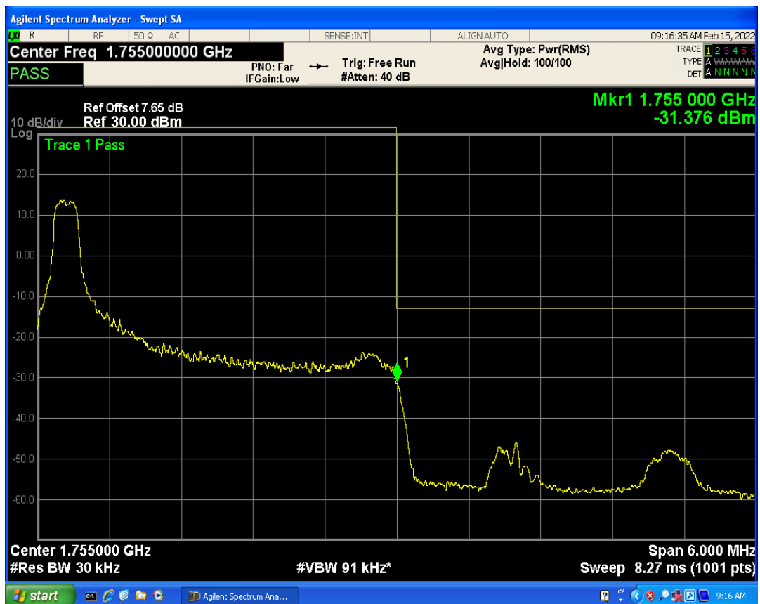
Band4 QAM16 BW=3MHz Channel=20385 RB Size=15 Position=#0
