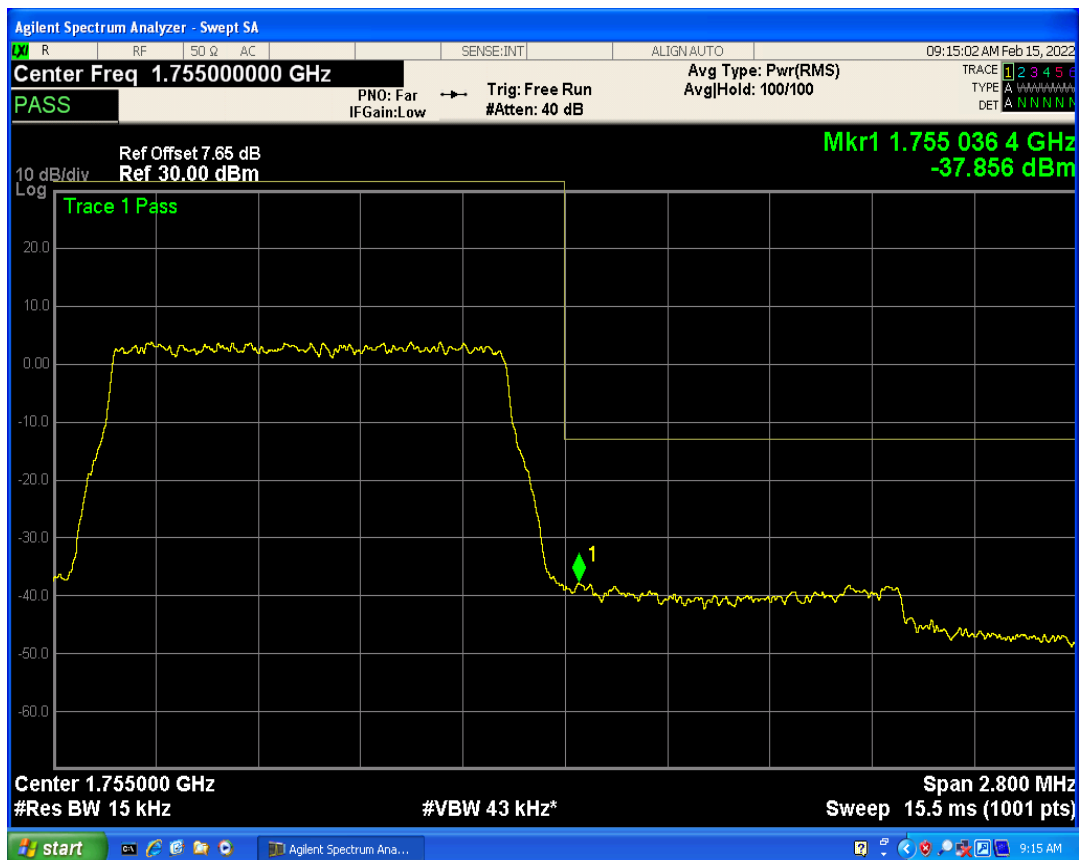
Band4 QAM16 BW=1.4MHz Channel=20393 RB Size=1 Position=#Max
