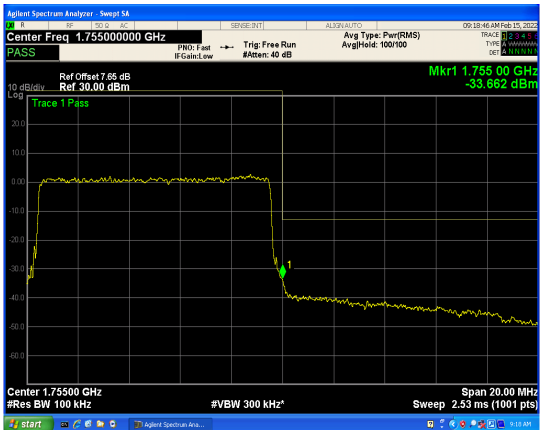
Band4 QPSK BW=15MHz Channel=20025 RB Size=1 Position=#Max
