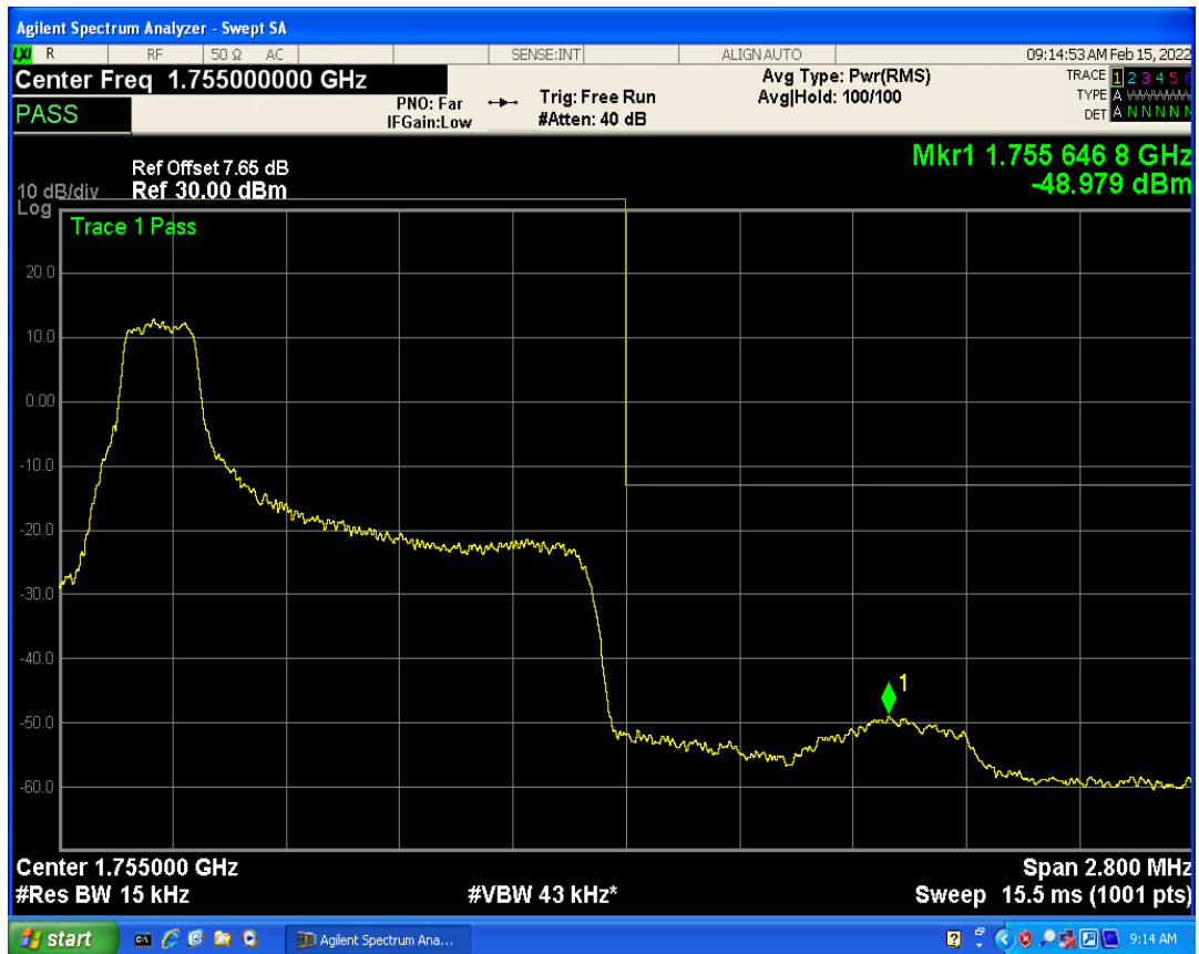
Band4 QPSK BW=1.4MHz Channel=20393 RB Size=1 Position=#Max
