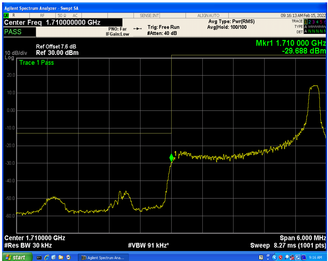
Band4 QPSK BW=3MHz Channel=20385 RB Size=1 Position=#0
