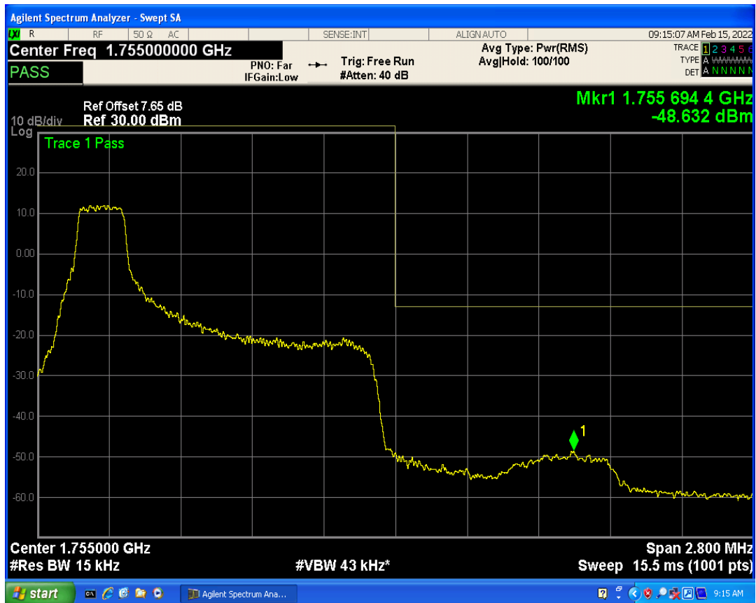
Band4 QPSK BW=1.4MHz Channel=20393 RB Size=6 Position=#0
