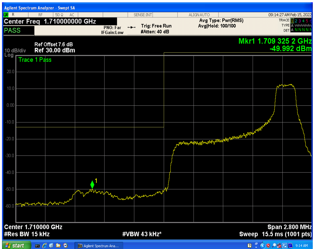
Band4 QPSK BW=1.4MHz Channel=19957 RB Size=6 Position=#0
