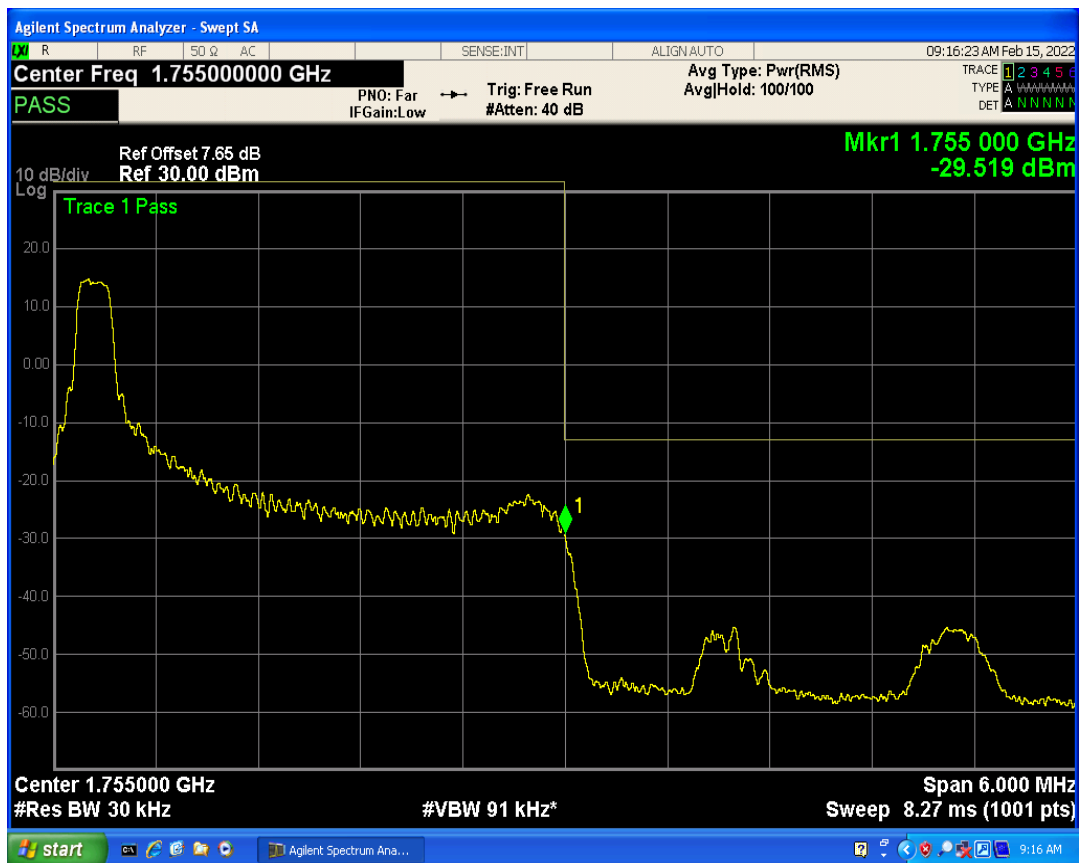
Band4 QPSK BW=3MHz Channel=20385 RB Size=15 Position=#0
