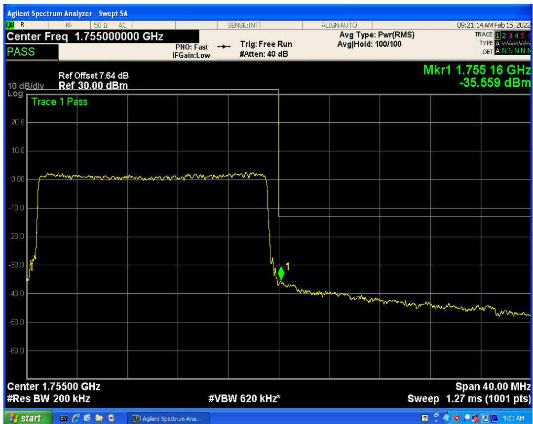
Band7 QPSK BW=5MHz Channel=20775 RB Size=1 Position=#0
