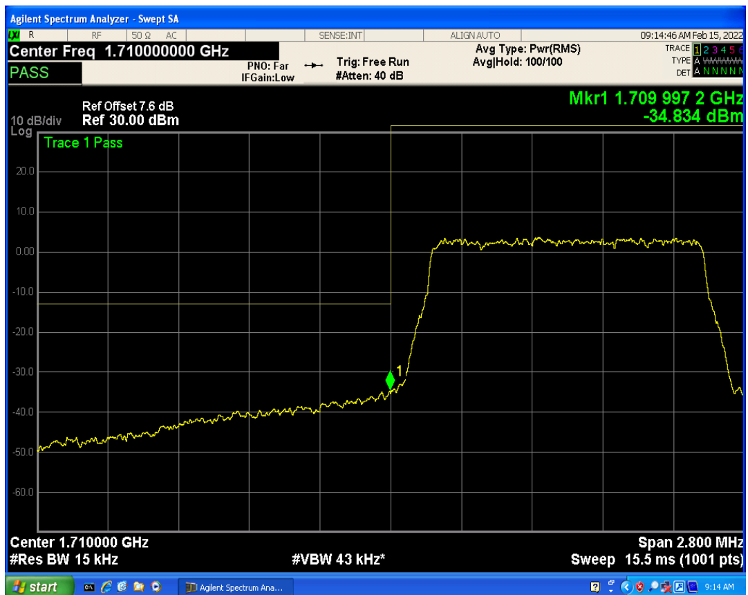
Band4 QPSK BW=1.4MHz Channel=20393 RB Size=1 Position=#0
