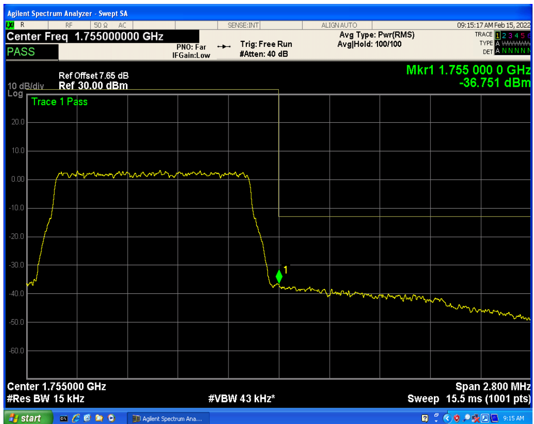
Band4 QPSK BW=3MHz Channel=19965 RB Size=1 Position=#Max
