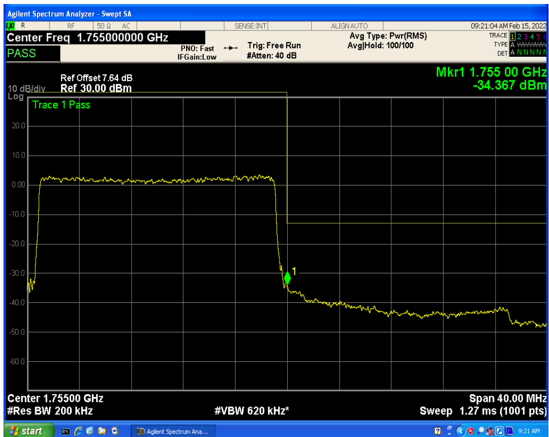
Band4 QPSK BW=20MHz Channel=20300 RB Size=1 Position=#Max
