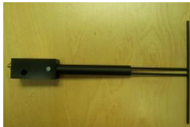
Figure 1 – MVG COMOSAR Validation Dipole
