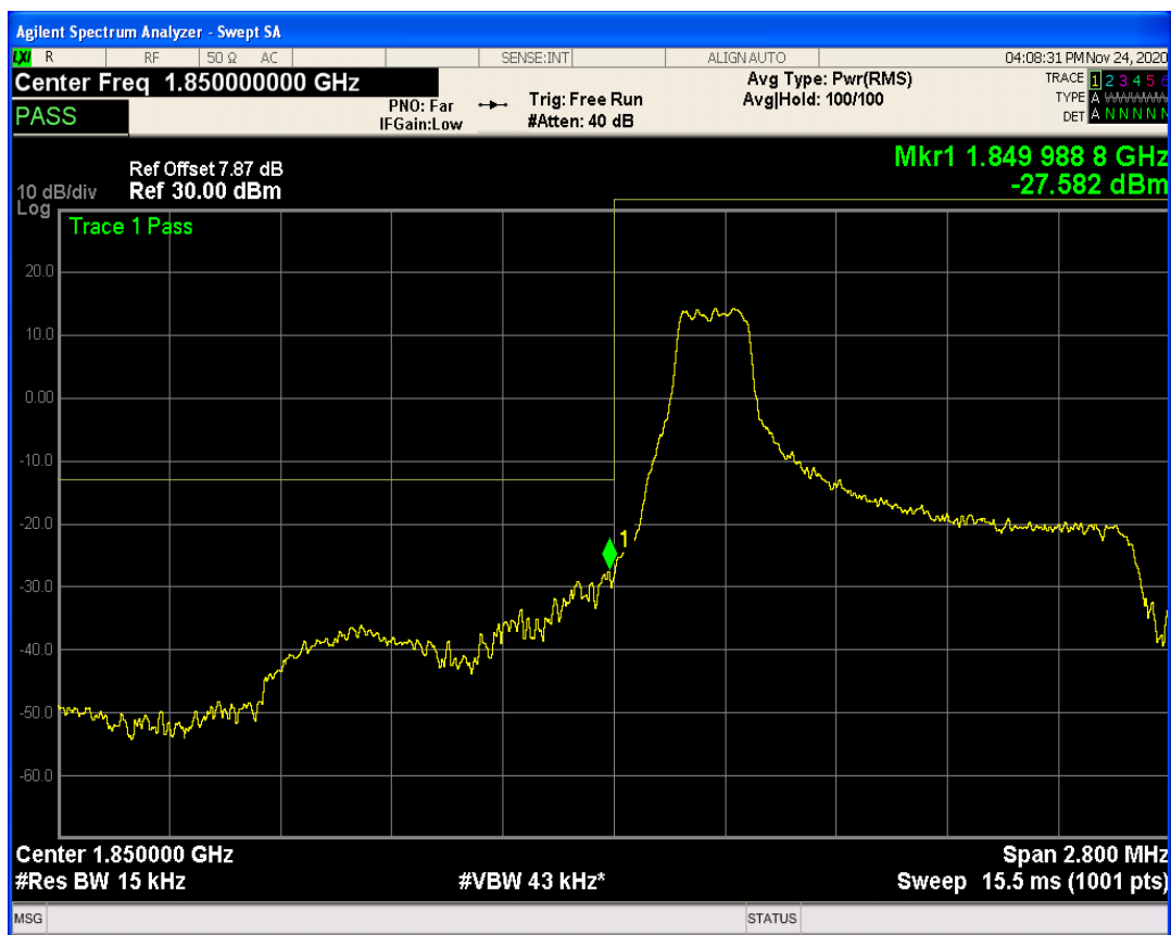
Band2 QAM16 BW=1.4MHz Channel=18607 RB Size=1 Position=#Max
