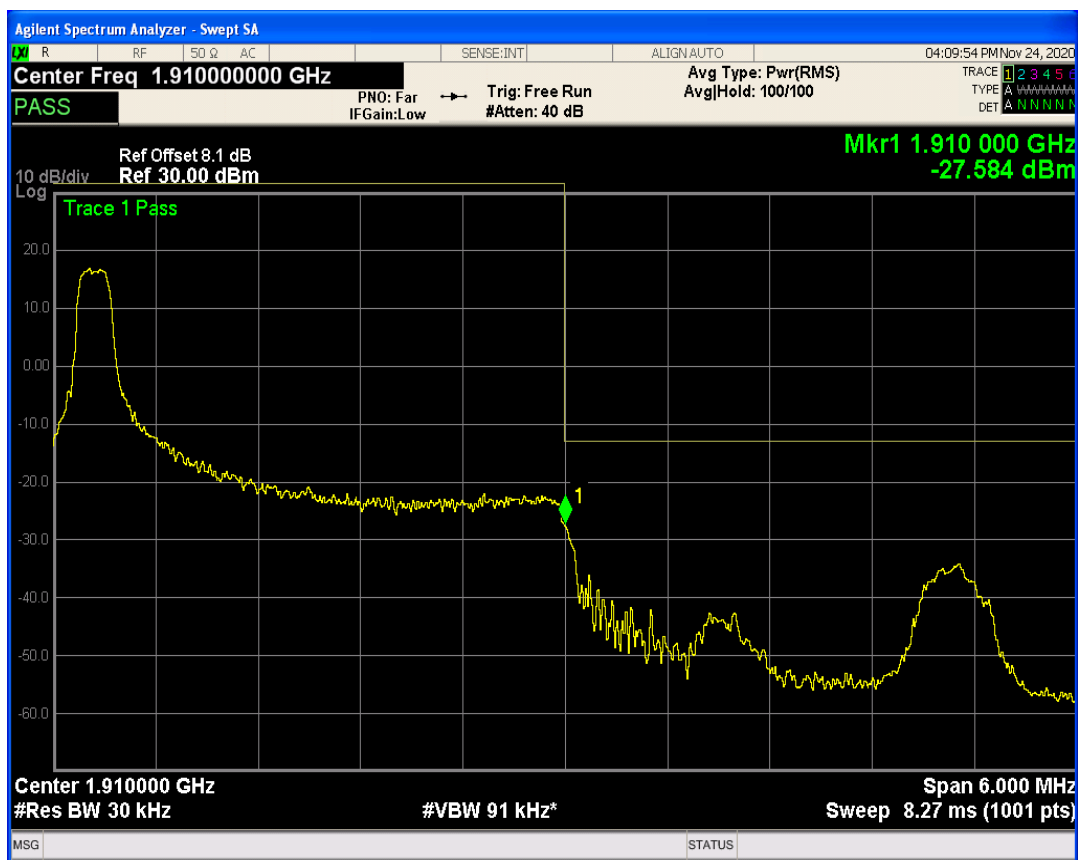
Band2 QPSK BW=3MHz Channel=19185 RB Size=15 Position=#0
