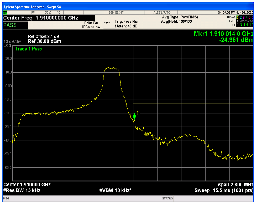
Band2 QPSK BW=3MHz Channel=18615 RB Size=1 Position=#0
