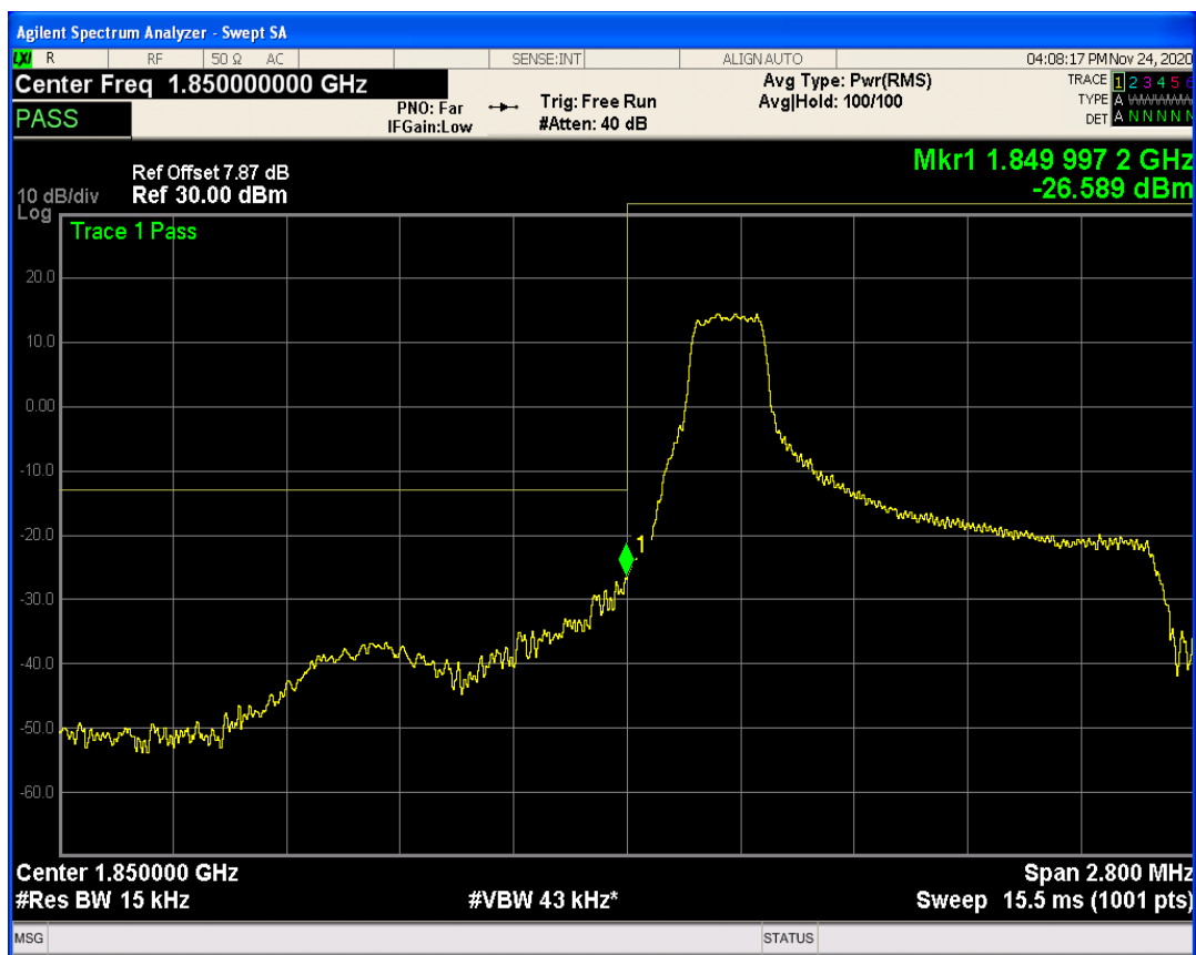
Band2 QPSK BW=1.4MHz Channel=18607 RB Size=6 Position=#0
