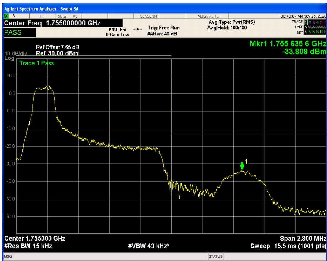
Band4 QAM16 BW=1.4MHz Channel=20393 RB Size=1 Position=#Max
