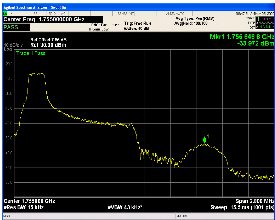
Band4 QAM16 BW=1.4MHz Channel=19957 RB Size=6 Position=#0
