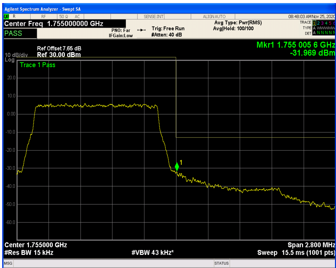
Band4 QAM16 BW=1.4MHz Channel=20393 RB Size=1 Position=#0
