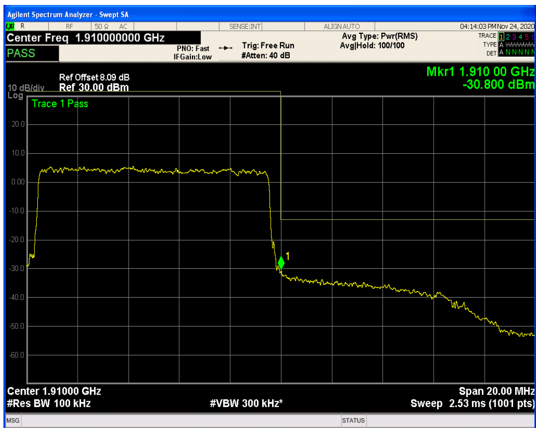
Band2 QAM16 BW=10MHz Channel=19150 RB Size=1 Position=#0
