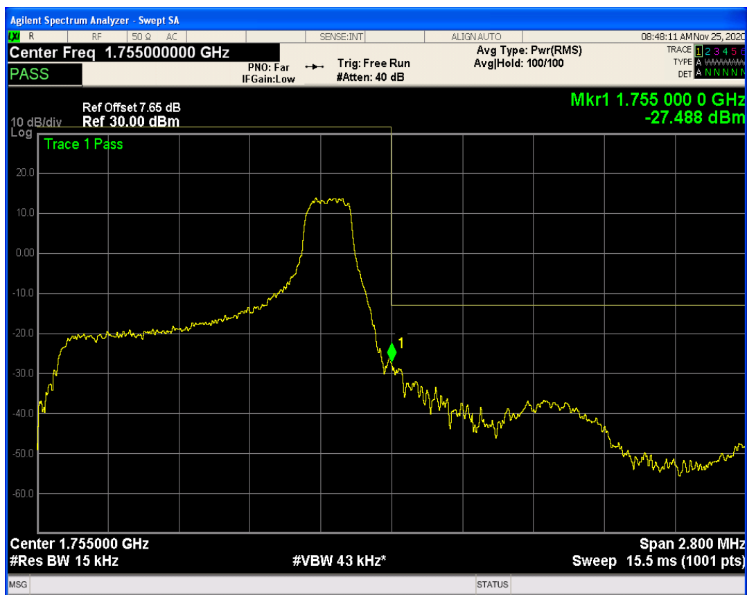
Band4 QPSK BW=3MHz Channel=19965 RB Size=1 Position=#0
