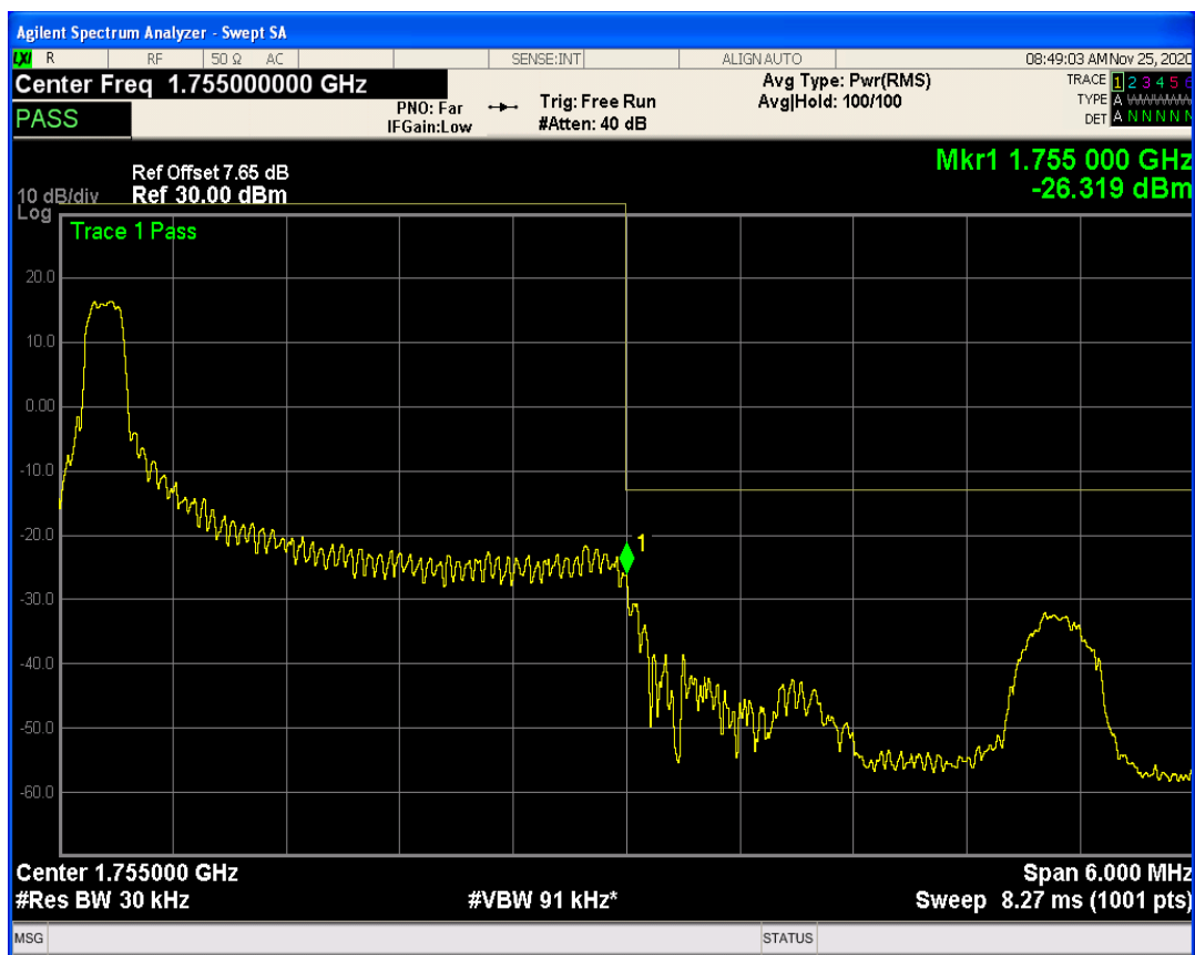
Band4 QAM16 BW=3MHz Channel=20385 RB Size=1 Position=#Max
