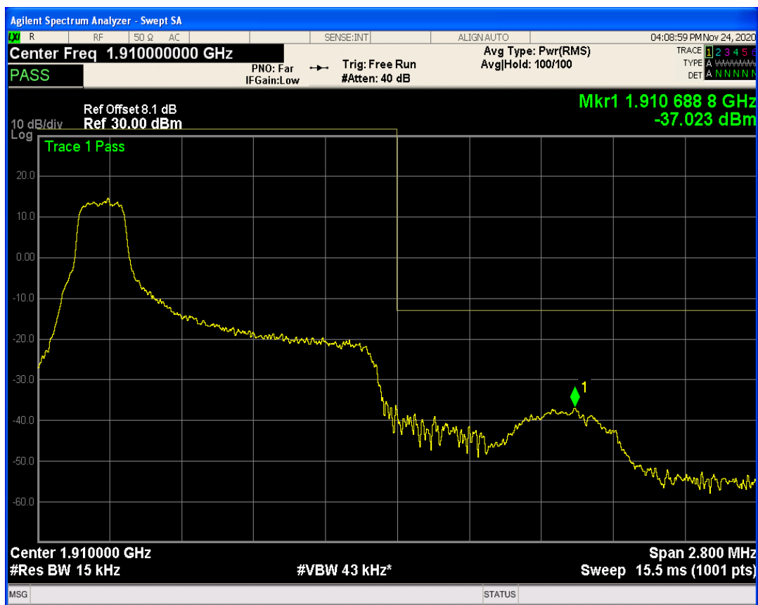
Band2 QAM16 BW=1.4MHz Channel=19193 RB Size=1 Position=#Max
