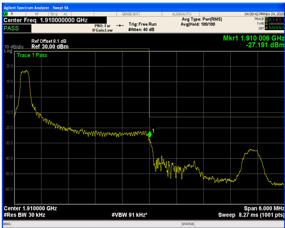
Band2 QAM16 BW=3MHz Channel=18615 RB Size=15 Position=#0
