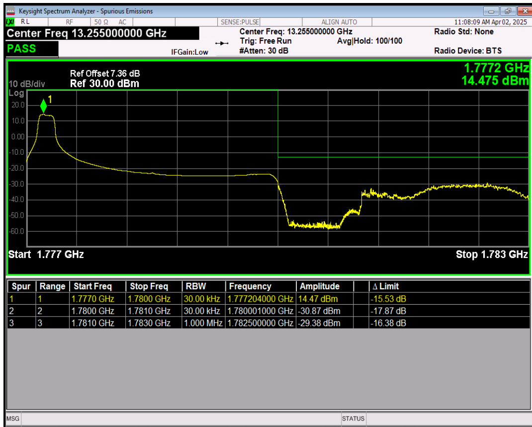
Band66 16QAM BW=3MHz Channel=132657 RB Size=1 Position=#Max
