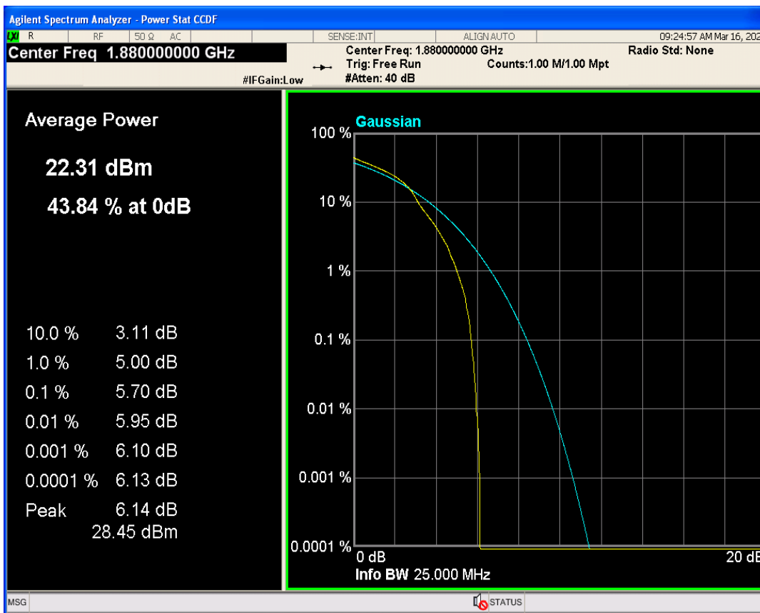
Band2 QAM16 BW=3MHz Channel=18900 RB Size=1 Position=#0
