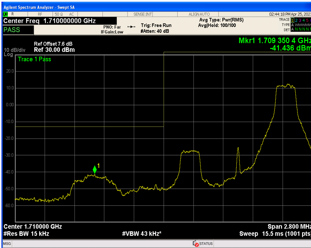
Band4 QPSK BW=1.4MHz Channel=19957 RB Size=6 Position=#0
