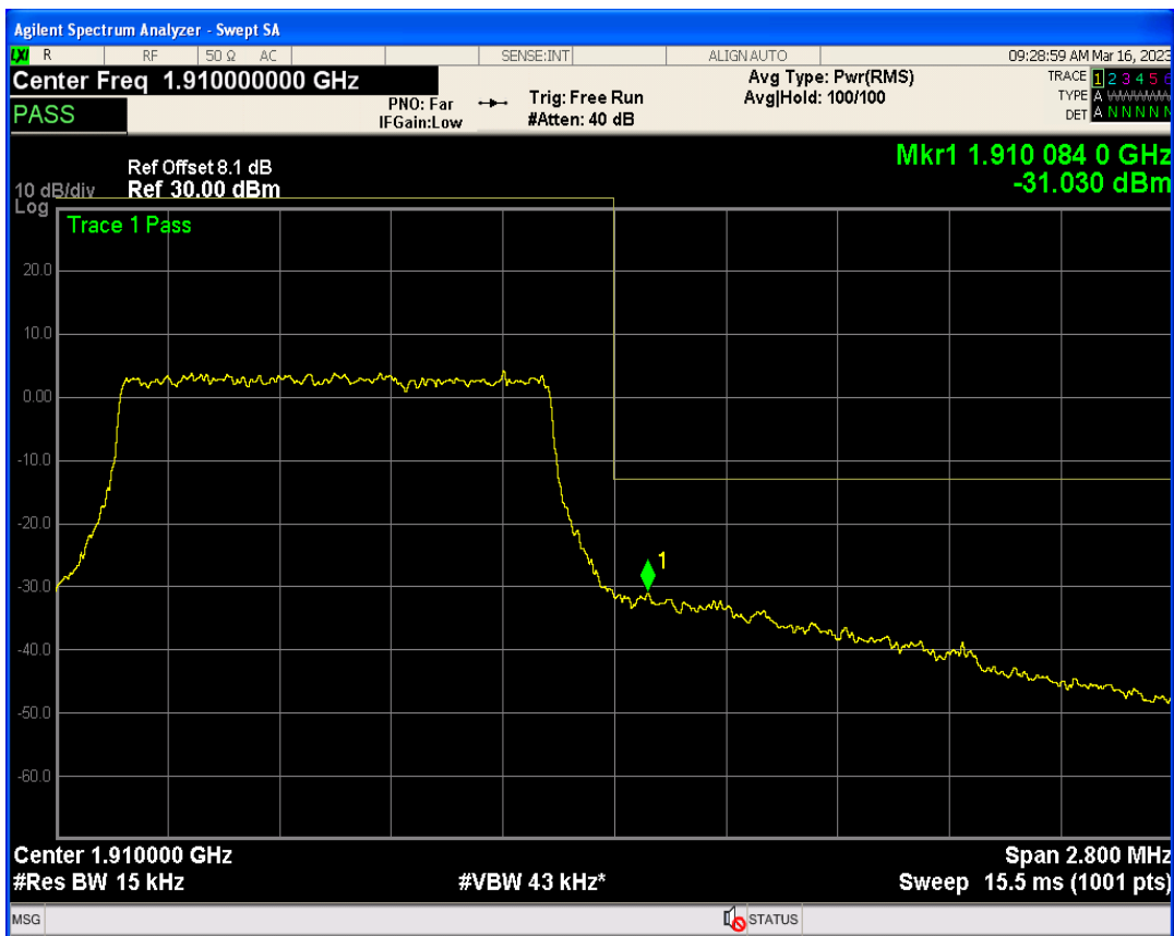
Band2 QPSK BW=3MHz Channel=18615 RB Size=1 Position=#Max
