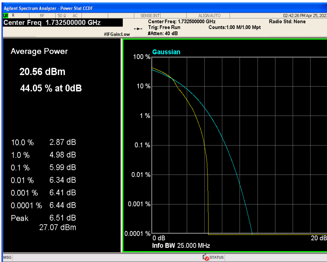
Band4 QPSK BW=10MHz Channel=20175 RB Size=1 Position=#0
