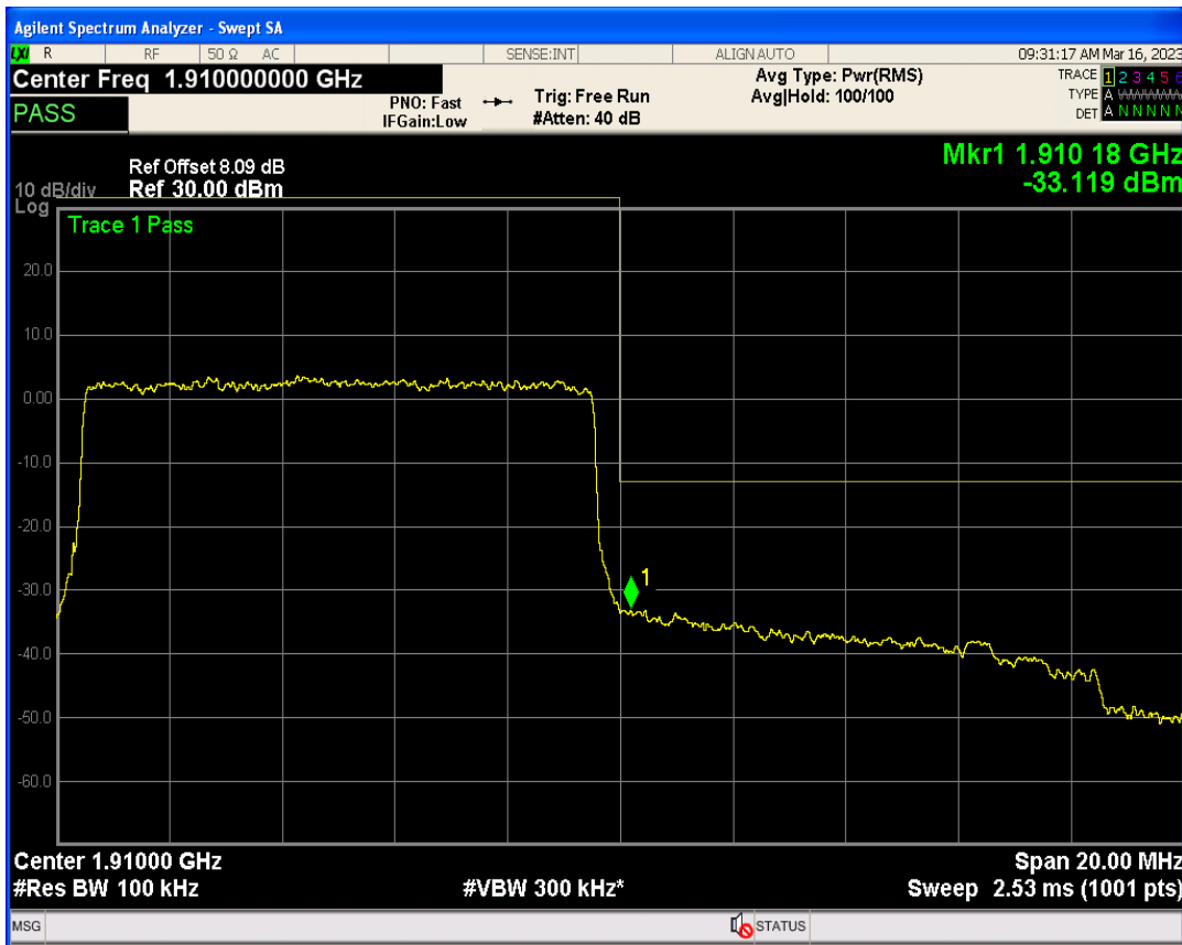
Band2 QAM16 BW=10MHz Channel=19150 RB Size=1 Position=#0
