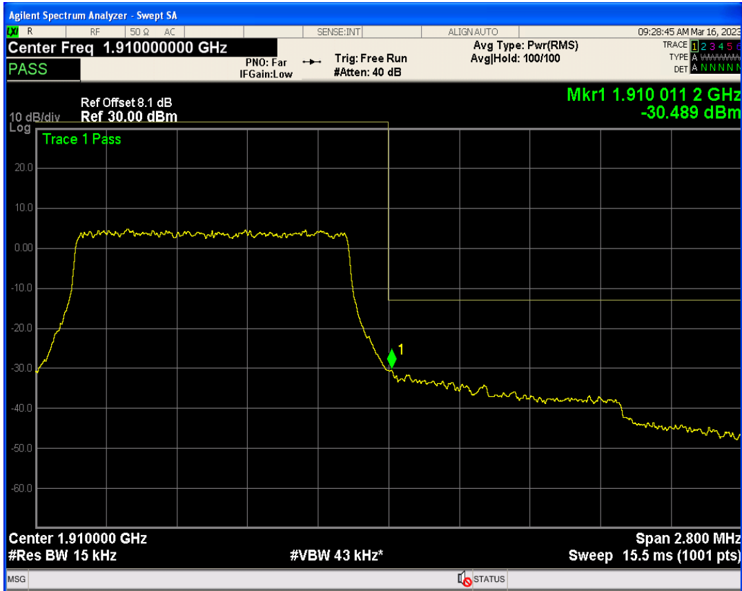
Band2 QAM16 BW=1.4MHz Channel=19193 RB Size=1 Position=#0
