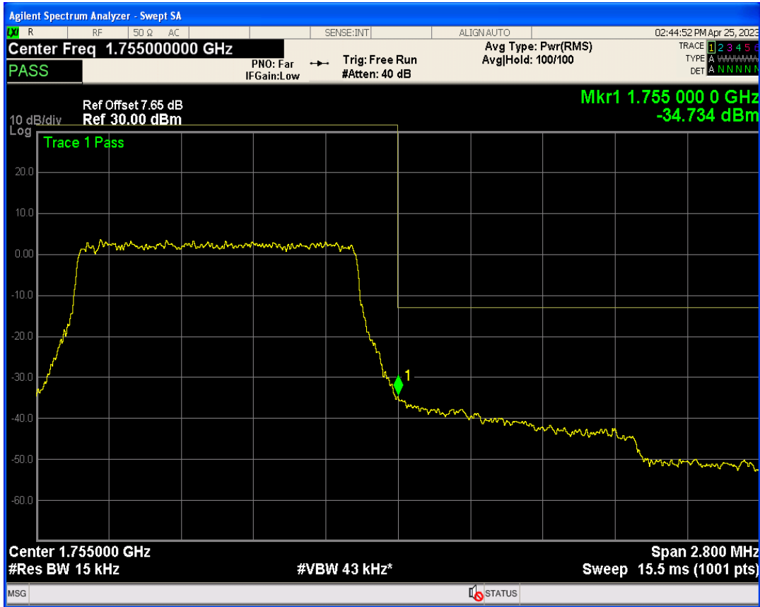
Band4 16QAM BW=1.4MHz Channel=20393 RB Size=1 Position=#0
