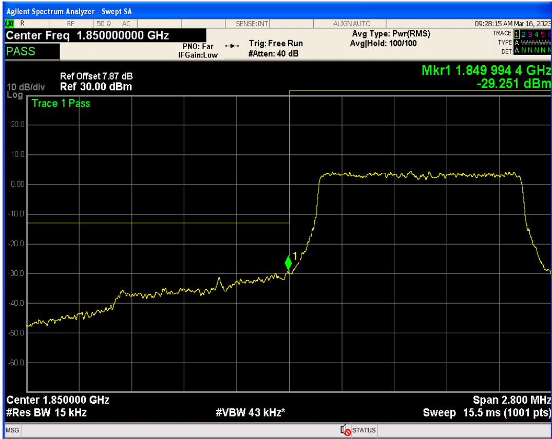
Band2 QAM16 BW=1.4MHz Channel=18607 RB Size=1 Position=#0
