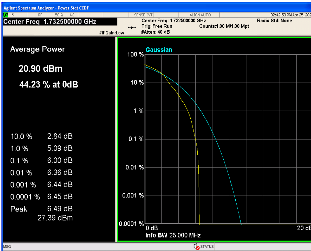
Band4 16QAM BW=20MHz Channel=20175 RB Size=1 Position=#0
