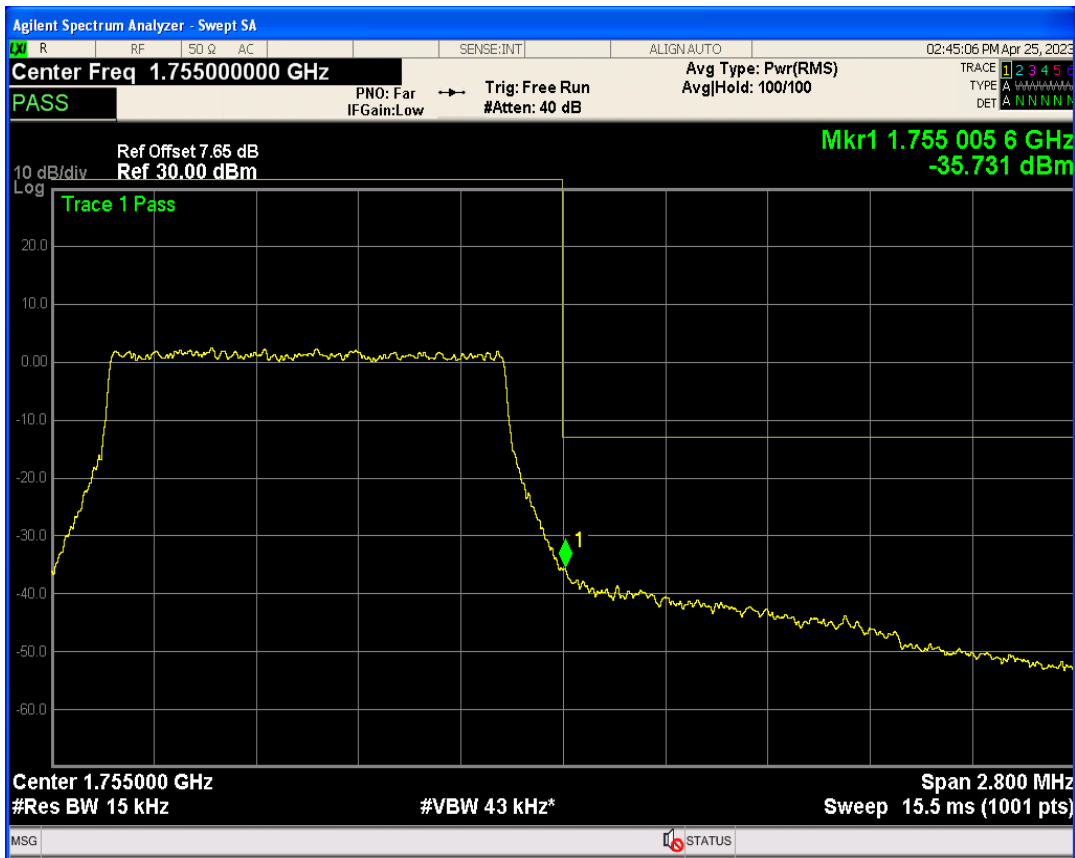
Band4 QPSK BW=3MHz Channel=19965 RB Size=1 Position=#Max
