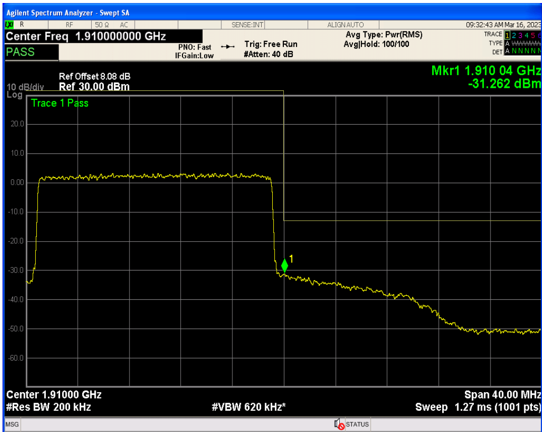
Band2 QAM16 BW=20MHz Channel=19100 RB Size=1 Position=#0
