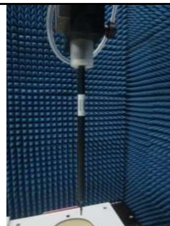
Fig.8.2 Photo of E-Field Probe
