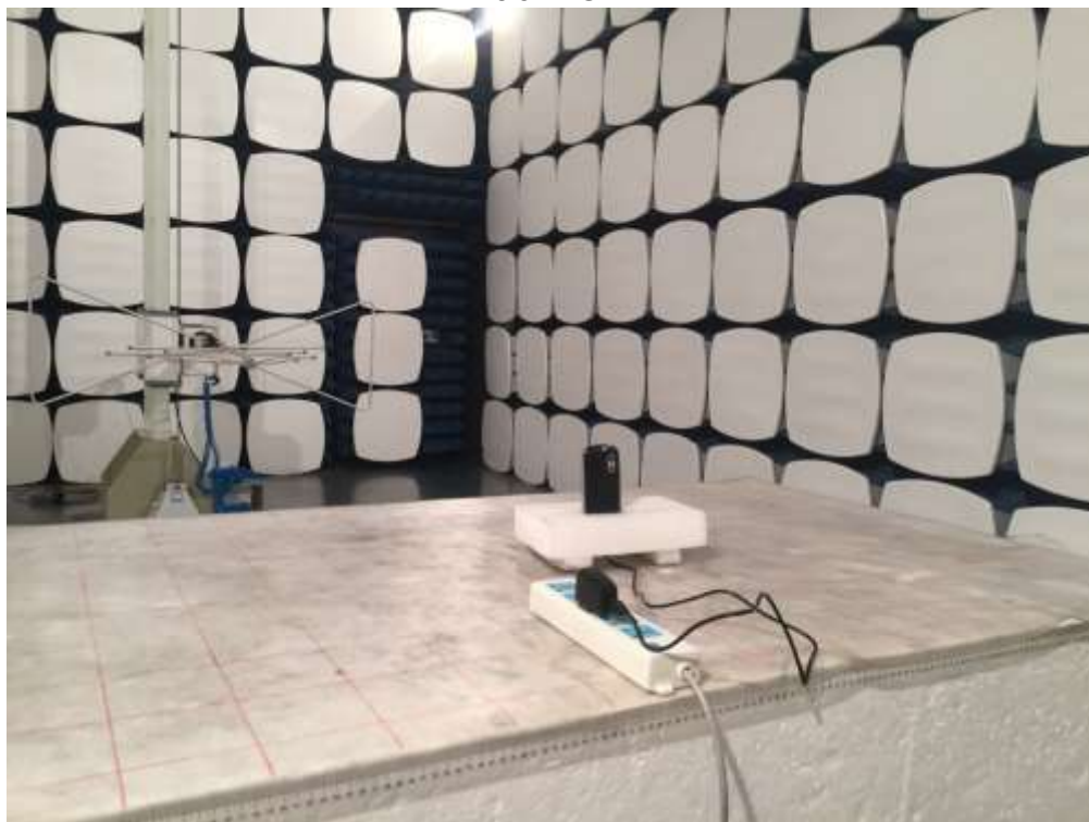
Radiated Spurious Emission Below 1GHz
