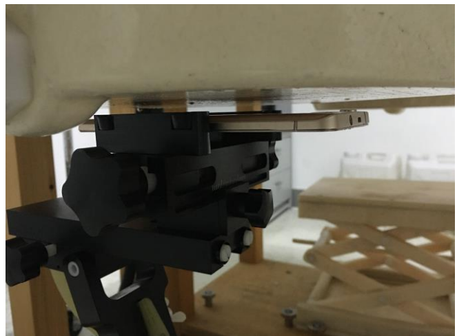
Back of the EUT with 1 cm Gap
