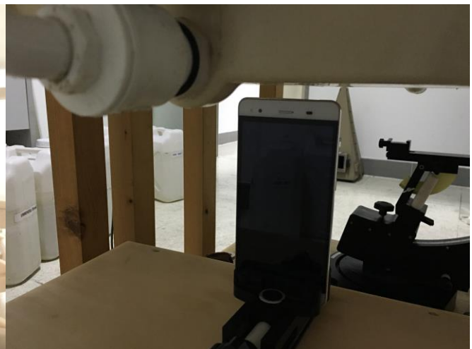
Top of the EUT with 1 cm Gap
