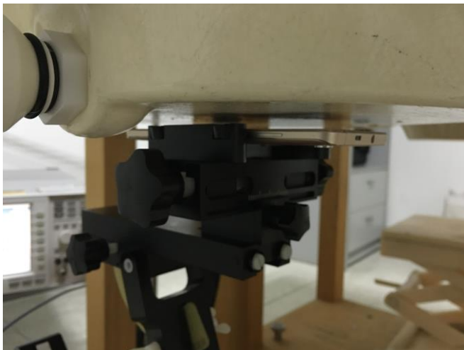
Front of the EUT with 1 cm Gap
