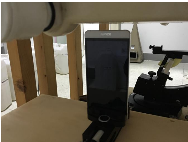
Bottom of the EUT with 1 cm Gap
