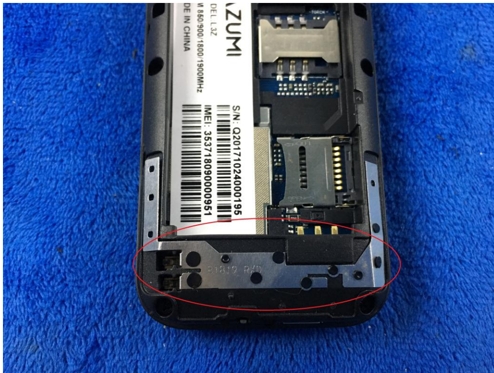
GSM/PCS Antenna View
