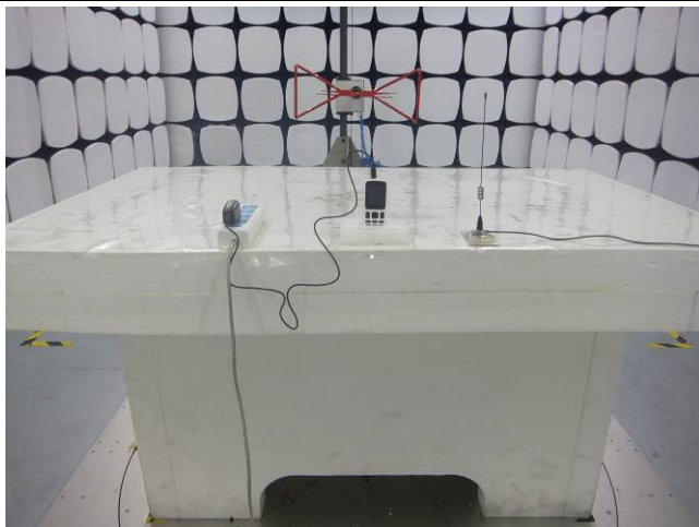
Radiated Emissions Test Setup Below 1GHz
