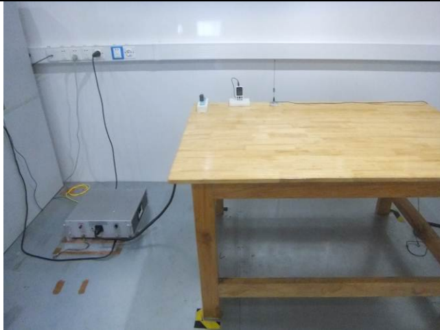
Conducted Emissions Test Setup Front View
