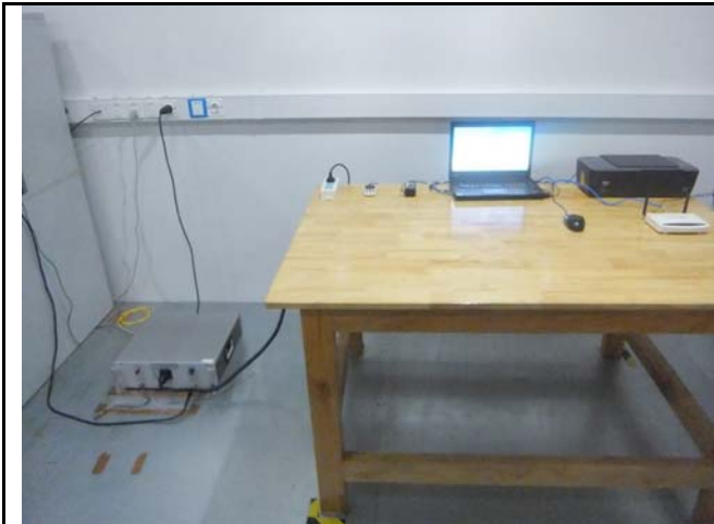
Conducted Emissions Test Setup – Front View
