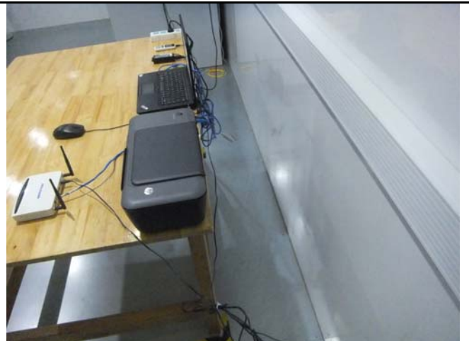
Conducted Emissions Test Setup – Side View
