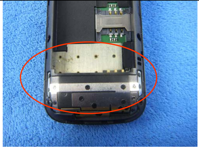
GSM/PCS/UMTS-FDD Antenna View
