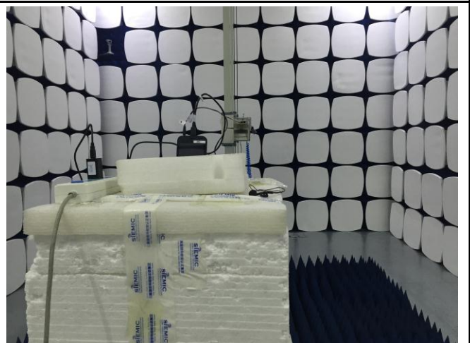
Radiated Spurious Emissions Test Setup Above 1GHz
