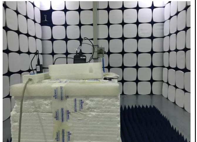
Radiated Spurious Emissions Test Setup Above 1GHz
