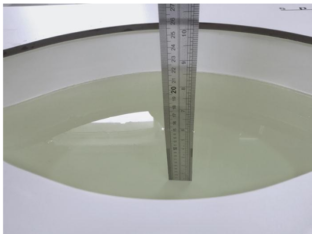
Liquid depth in the body phantom (2450MHz)
