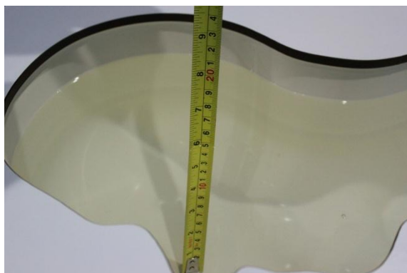
Liquid depth in the head phantom (2600MHz)
