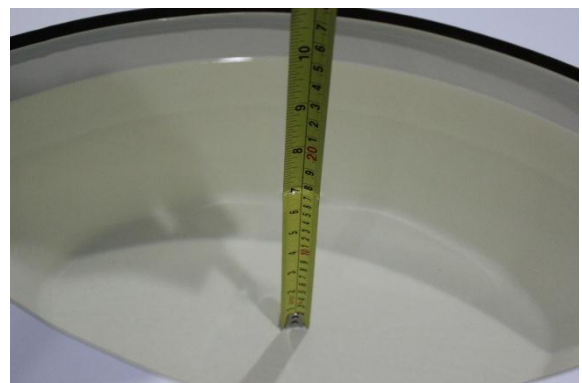
Liquid depth in the body phantom (2600MHz)
