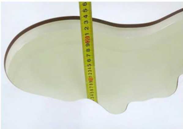
Liquid depth in the head phantom (835MHz)
