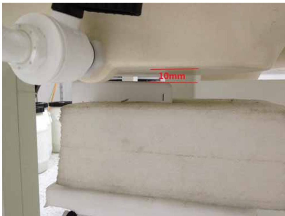
Body Left side at 10mm WLAN
