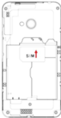
Please insert the SIM card(s) according to the label on the phone. Make sure that the clipped corner of the SIM card and the metallic contacts are facing the correct direction. Slide the SIM card into the slot until it doesn't move up any further.
