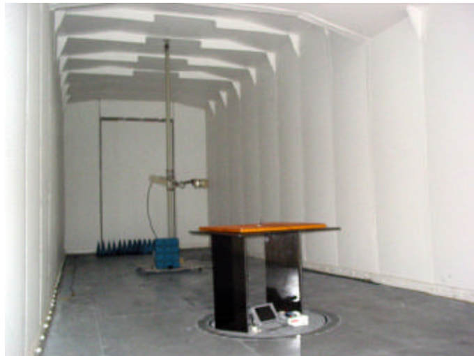
WaveCell Neptune WEX-10 CDPD Modem tested for Spurious Emissions from Transmitter Frequency Range: 1 GHz – 18 GHz
