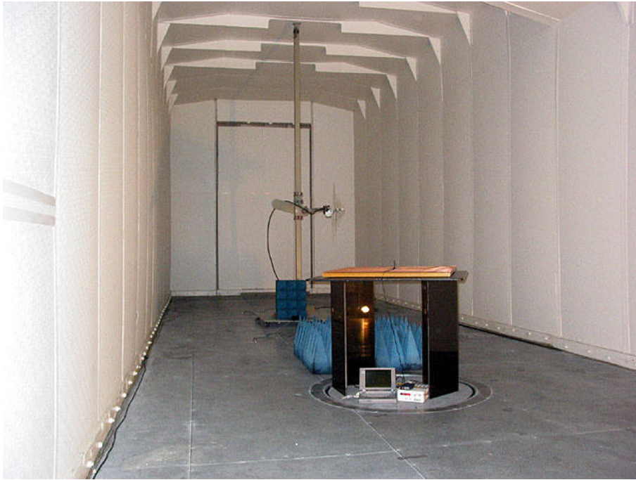
WaveCell Neptune Wex-10 CDPD Modem set up for ERP measurement The equipment is under the table and the antenna is mounted on the ground plane
