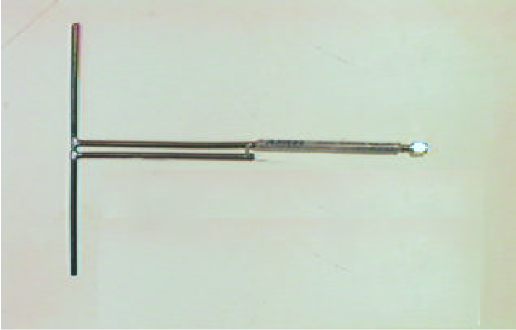
Reference Dipole Antenna Used for ERP Measurement
