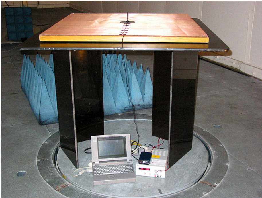
WaveCell Neptune Wex-10 CDPD Modem tested for ERP (Close View)
