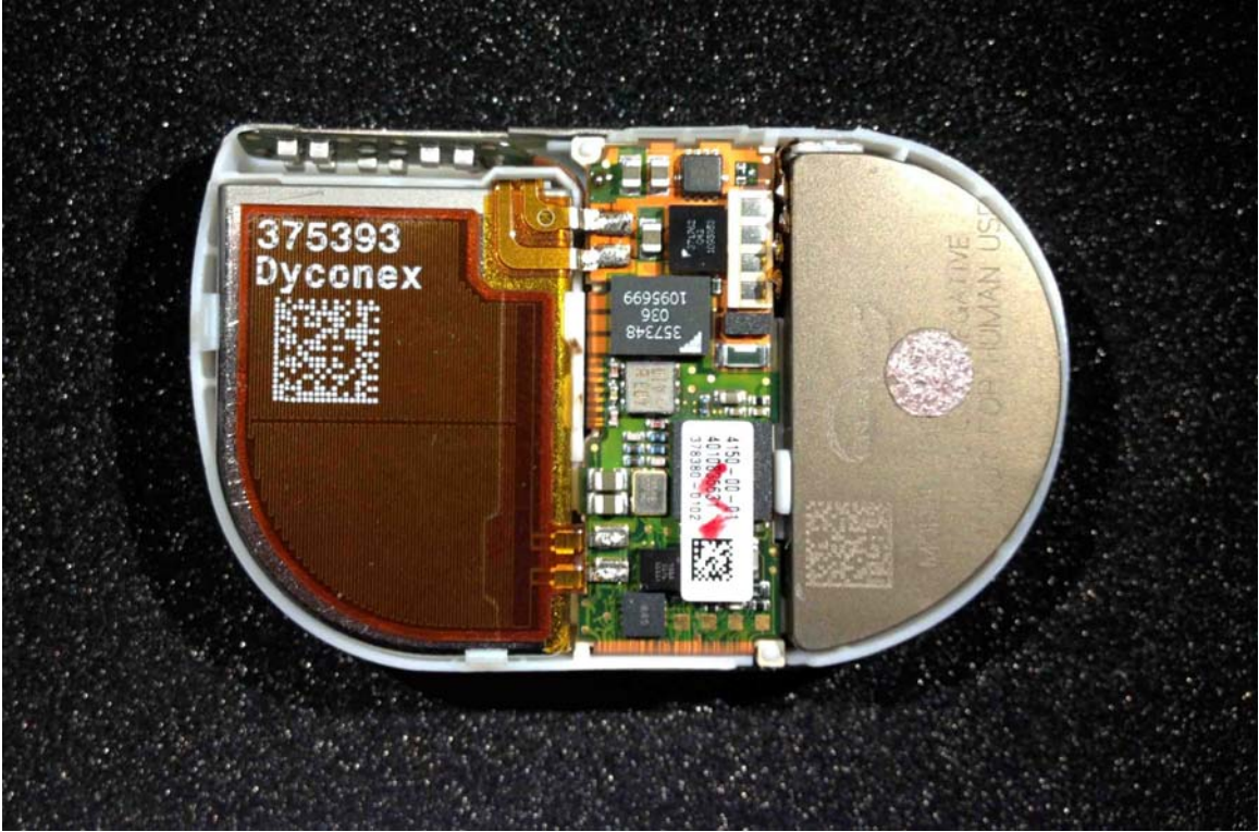
DUT - electronic module with mounting frame placed in half can with battery (left) and HV cap's (right) – top view
