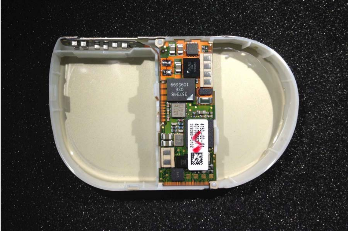
DUT - electronic module with mounting frame placed in half can – top view
