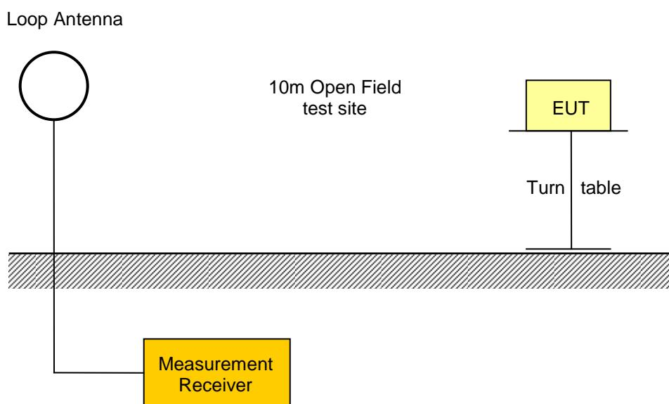
The eut is placed on a non-metallic table. Any emission is received by a loop antenna and measured via a measurement receiver connected to the loop antenna. To obtain the maximum emission the eut is rotated through 360°.
