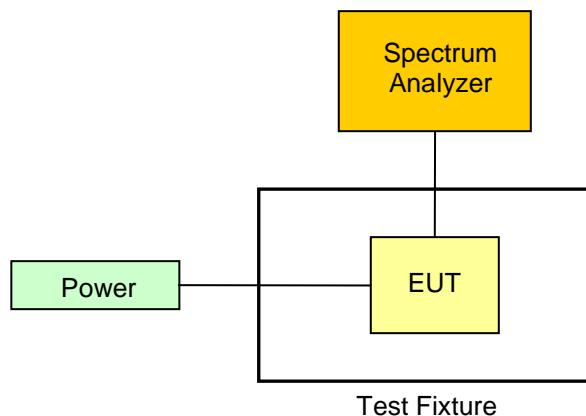
The eut is connected to a spectrum analyzer and set to transmission mode with maximum power under normal test conditions. The span of the analyzer is set wide enough to capture all significant emissions of the modulation spectrum. The resolutions bandwidth is set as close as possible to 1% of the selected span without being below 1%. The occupied bandwidth is than measured evaluated by an internal measurement procedure of the analyzer.
