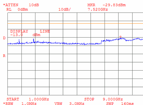
Plot 7.3.18 Spurious emission measurements in 1000 - 9000 MHz range at mid carrier frequency
