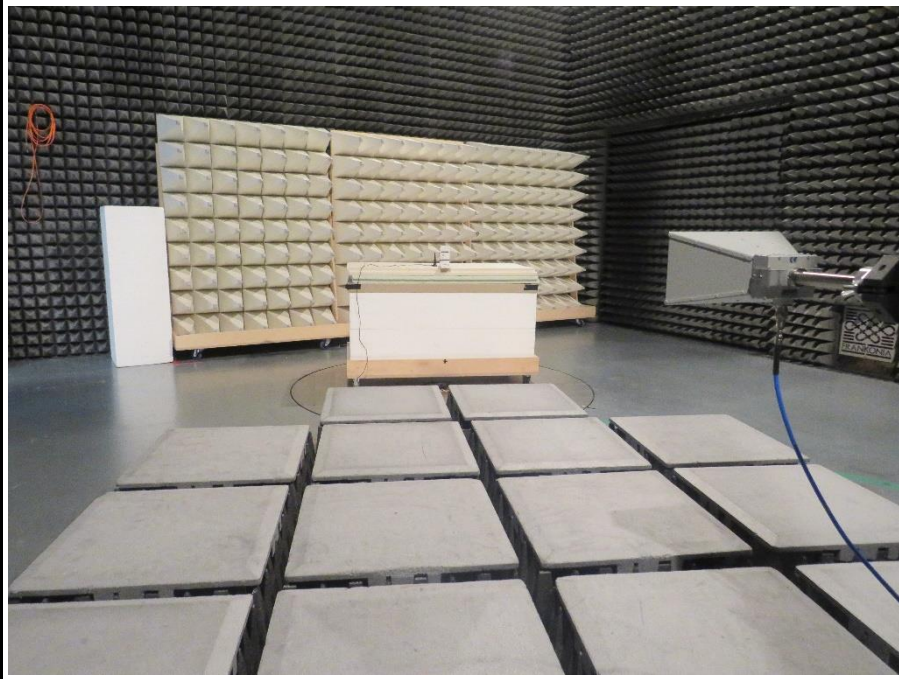
Test Setup radiated emissions idle mode above 1 GHz
