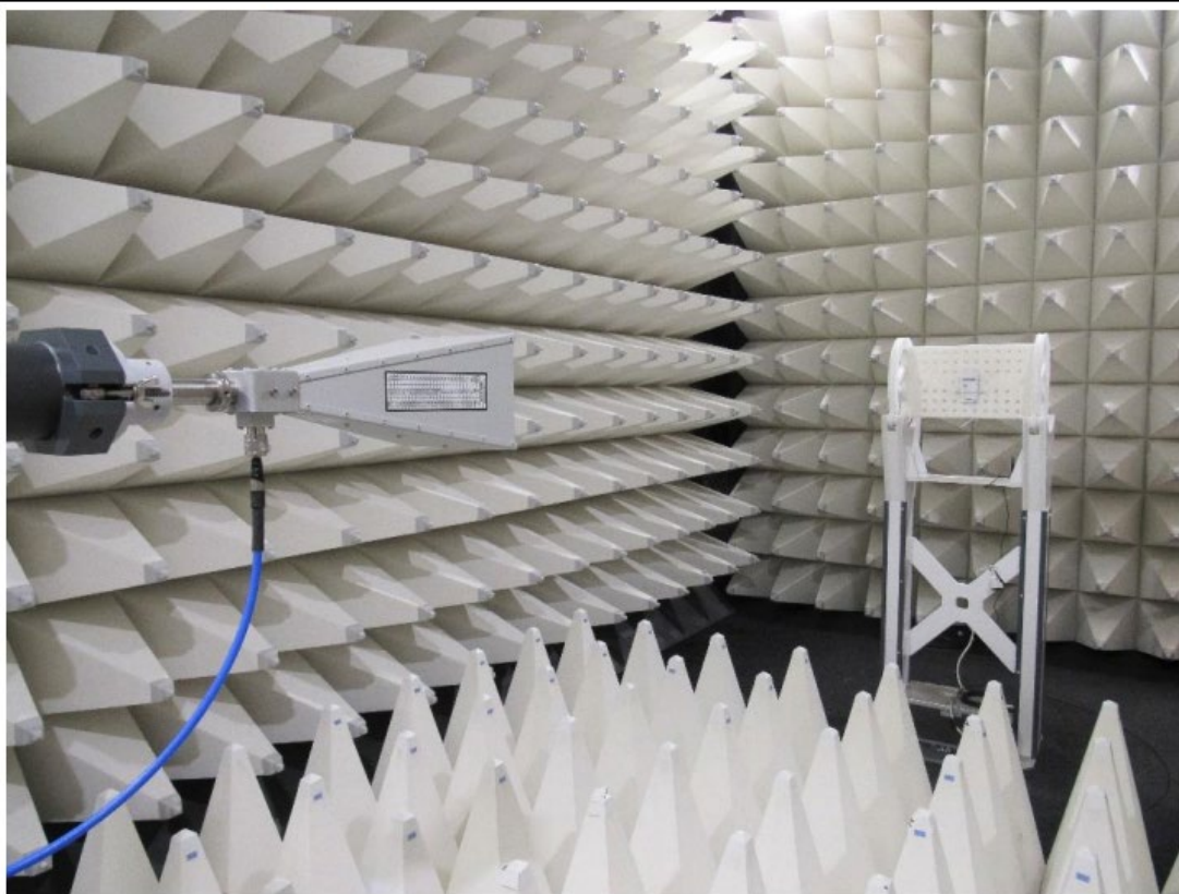
Test Setup radiated emissions transmit mode above 1 GHz
